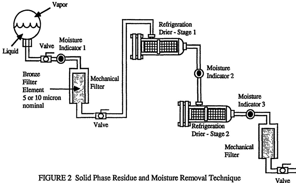
FIGURE 2 Solid Phase Residue and Moisture Removal Technique
