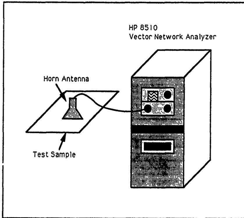
Figure 6: RAM Measurement Using A Vector Network Analyzer
