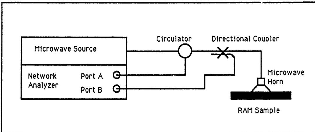
Figure 4: A Scalar Network Analyzer used for Reflection Measurements
