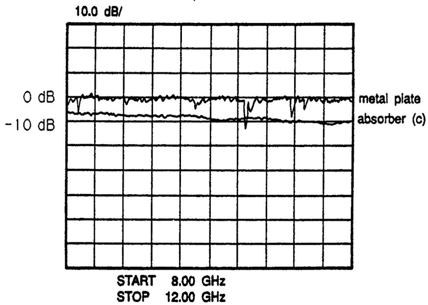
Figure 8: Comparison of reflected power from a Broadband Absorber and a Metal Plate vs. Frequency
