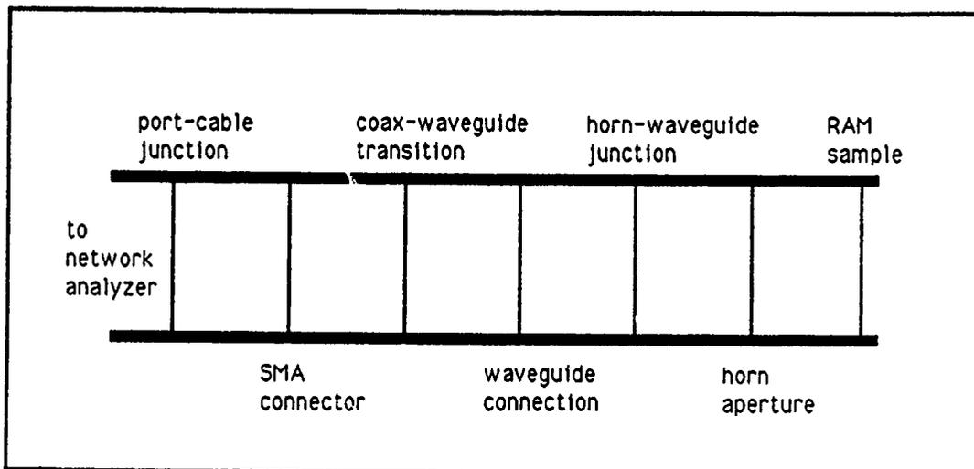
Figure 5: A Transmission Line Model of Discontinuities
