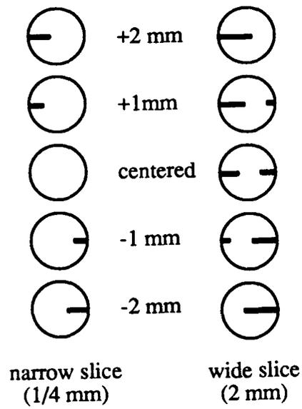
Figure 3.2-2 IQI images showing the centering indications.
