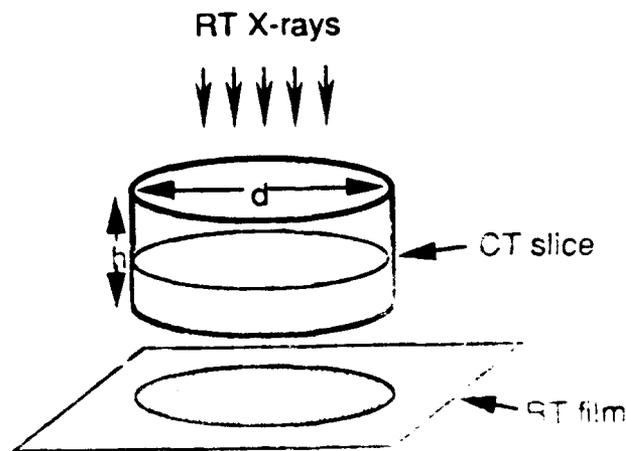
Figure 3.3-1 Example of RT and CT inspection of cylindrical object.
