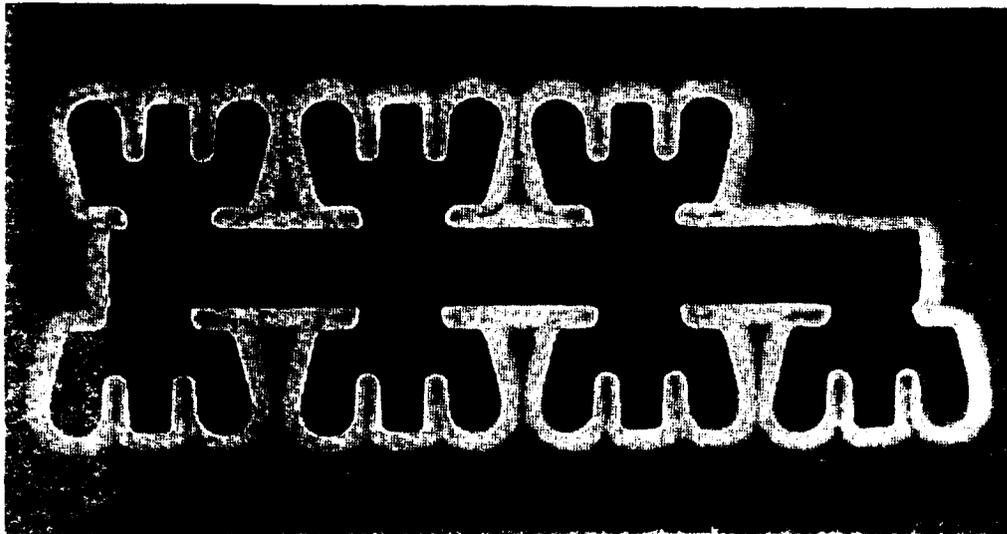
Figure 4.1-4 CT slice of the investment mold showing the inner layer (white) of zircon and the outer layer (gray) of silica.
