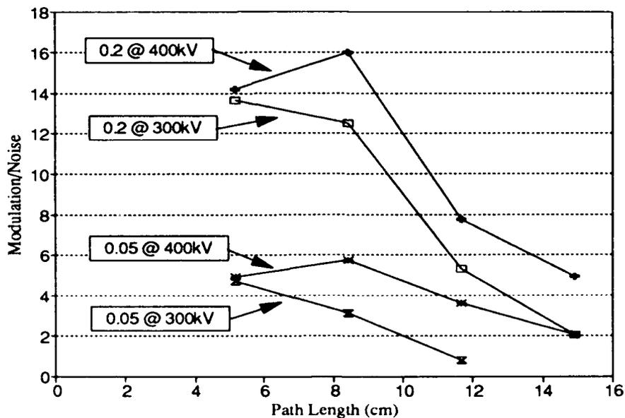
Figure 3.2-5 Modulation-to-noise ratio as a function of object size (path length) for voids of 0.2 and 0.05 mm<sup>3</sup> at 200 kV and 400 kV.
