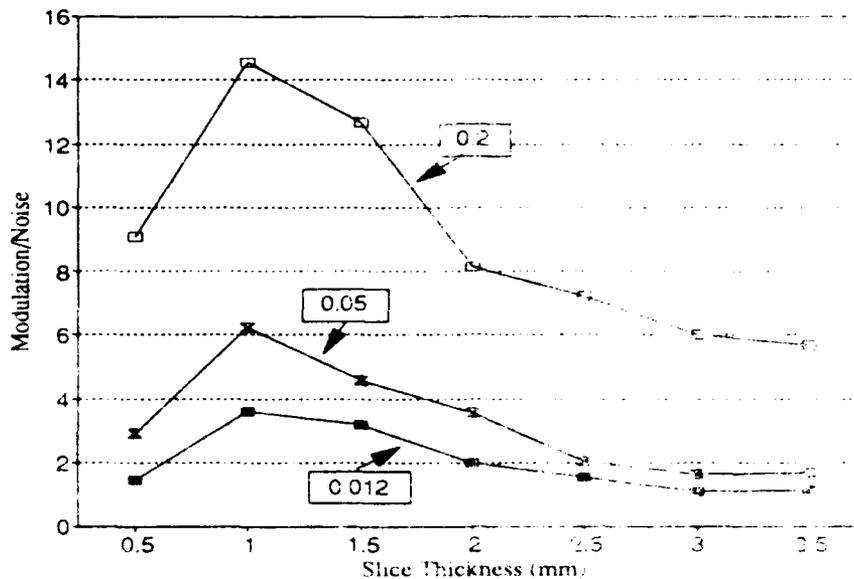
Figure 3.2-6 Modulation-to-noise ratio as a function of CT slice thickness for a 5 cm aluminum path length at 300 kV.
