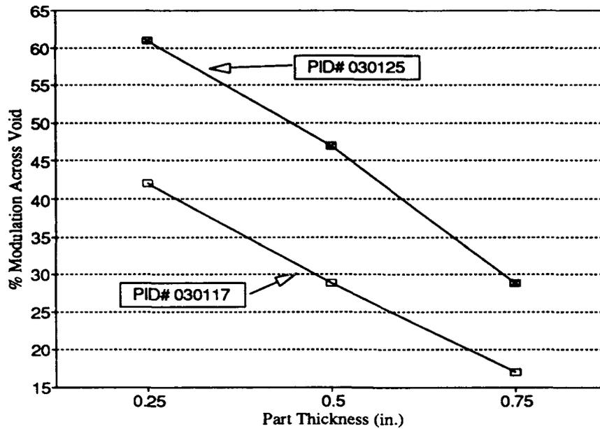
Figure 3.3-3 Graph showing the effect of thickness (path length) on RT defect sensitivity in cast coupons PID# 030117 and 030125.
