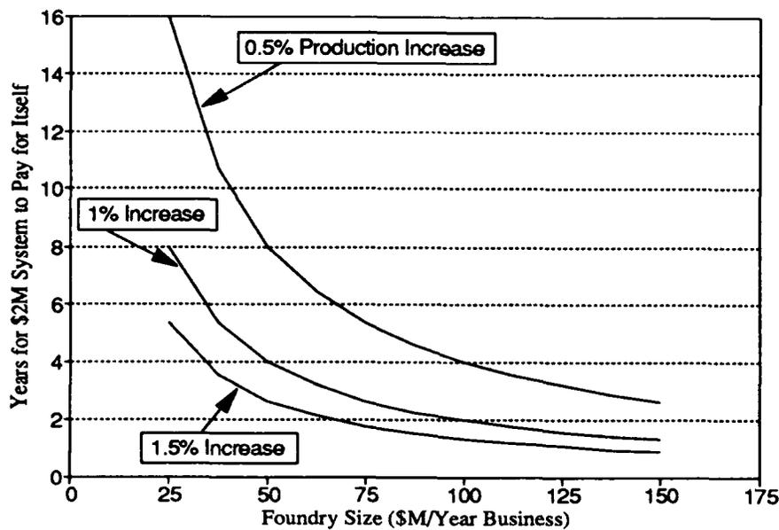
Figure 5.2-1 Estimated time for return on investment on a \$2M CT system if production were increased by 0.5, 1 or 1.5 percent (by reducing the scrap from 10 percent to 9.5, 9 and 8.5 percent respectively) in foundries of various size.
