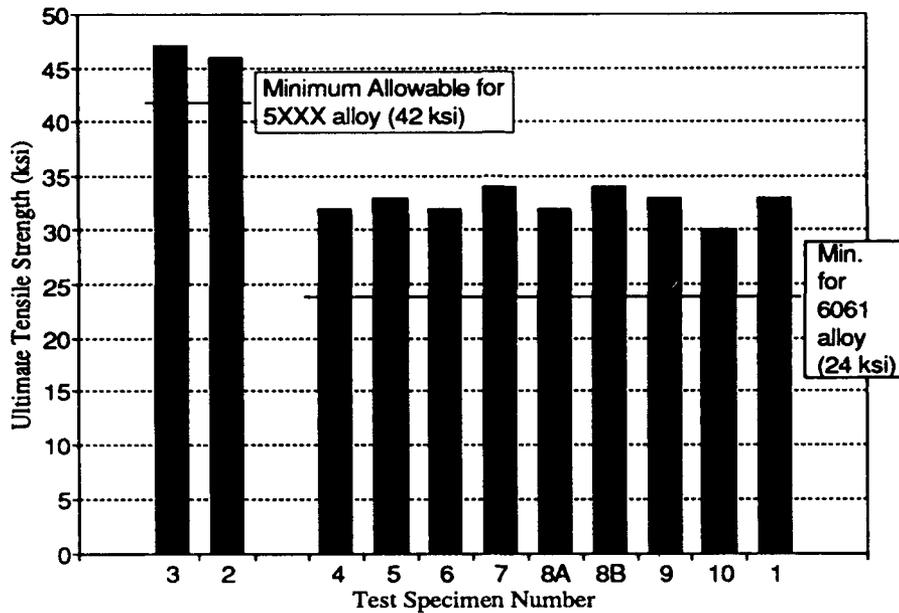
Figure 3.1-5 Welded Al test specimens with acceptable strength but rejectable radiographic porosity indications per BAC 5975, Class "A" or "B" welds.
