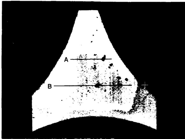
Figure 4.2-2 A digital radiograph (DR) of a section of the sector casting showing porosity. Some CT slice locations are indicated.
