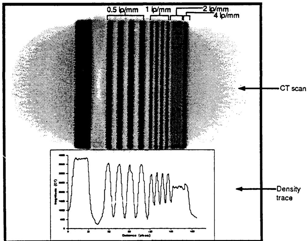
Figure B1-2 CT slice of the resolution phantom.
