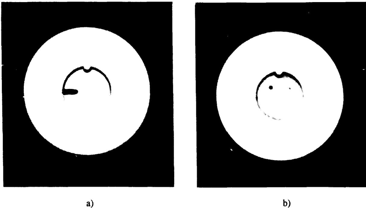
Figure 3.2-3 CT image of IQI with 0.25 mm slice a) located 1 mm high and b) centered on IQI.
