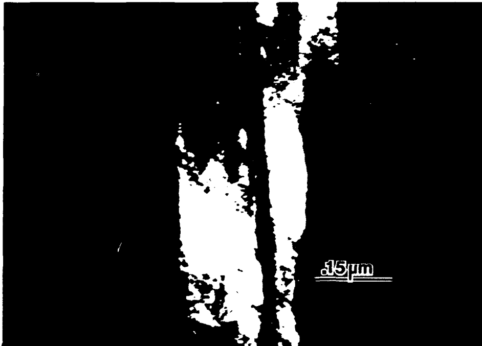
Figure 44. Dark Field TEM Micrograph of Lath Martensite Containing \epsilon -Copper Precipitates in HSLA-100 With Increased Copper Steel.
