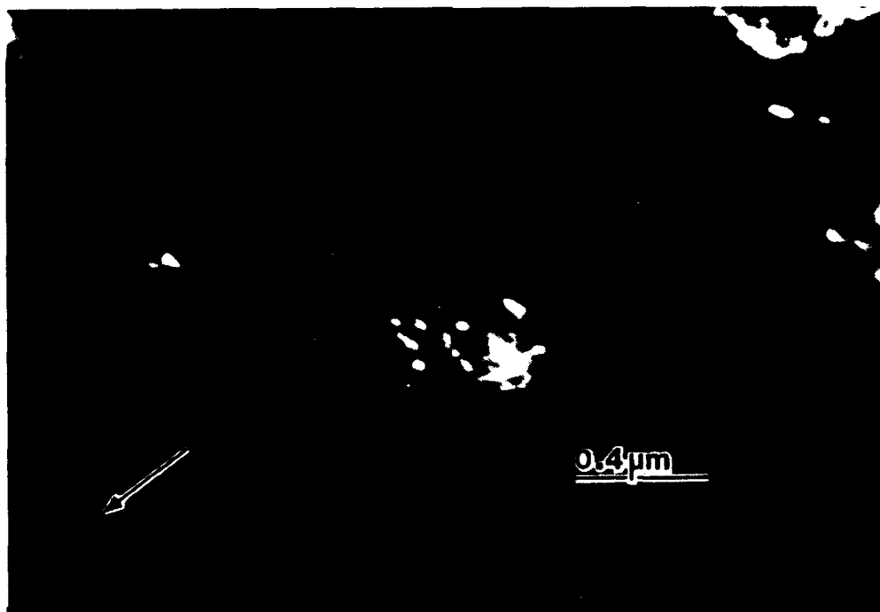
Figure 39. TEM Dark Field Image of Martensite Twinning in As-quenched HSLA-100 with Increased Copper Martensite Steel.
