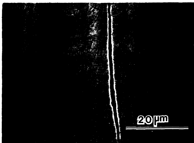
Figure 14. SEM Micrograph of a MnS Stringer in HSLA-100 with Increased Copper Steel.
