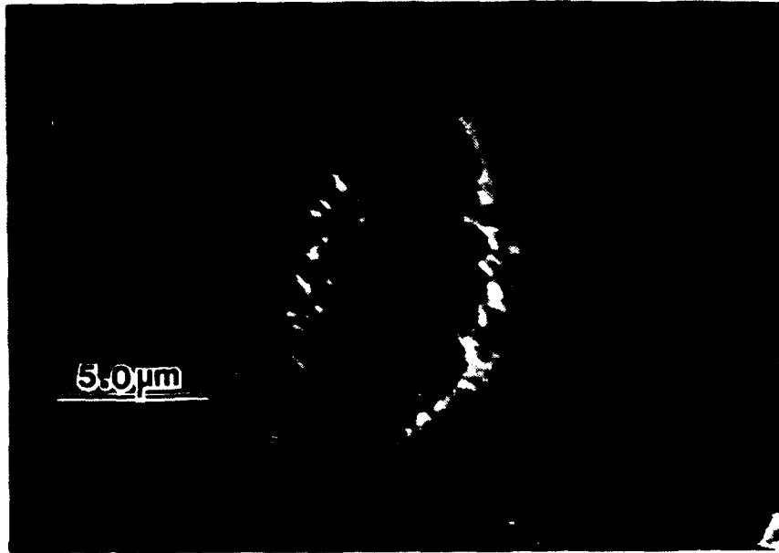
Figure 26. SEM Micrograph of an Oxy-Sulfide Inclusion in a ULCB Steel.
