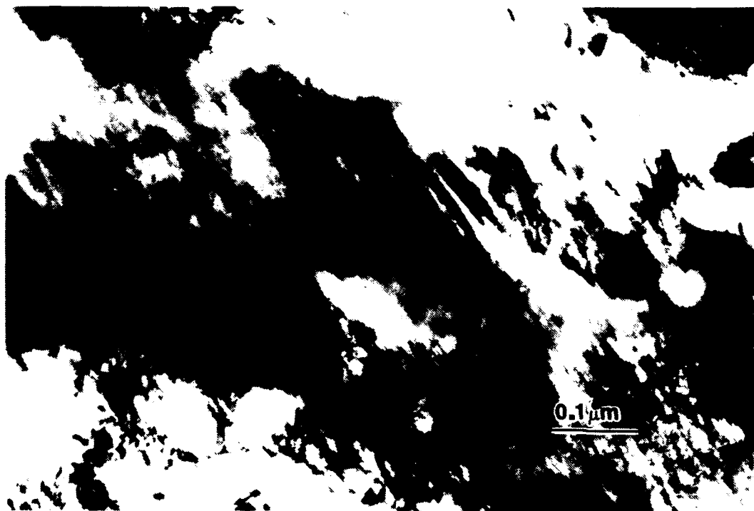
Figure 32. TEM Image of Twin Martensite in As-quenched HSLA-100 Steel.
