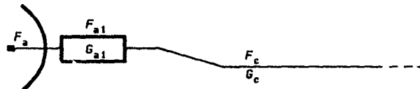
Figure 4. Antenna, amplifier, and cable.
