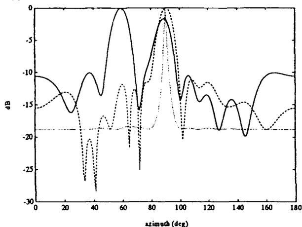
Figure 5: WVD DF on Two Chirps — One chirp at  $90^\circ$  azimuth sweeping down from 16 Hertz at -4 Hz/sec. The second chirp at  $60^\circ$  azimuth sweeping up from 0 Hertz at +4 Hz/sec. The solid line is the classical DF, the dashed line is classical WVD DF, and the dotted line is the MUSIC WVD DF (one signal).
