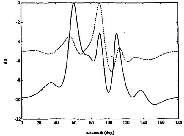
Figure 4: MVDR using a Gabor Prefilter — An 11-Hertz signal at 1/10 amplitude from  $90^\circ$  azimuth, additive  $\mathcal{N}(0,1)$  noise, and the five Gabor transients. The CSD was estimated at 11 Hertz by averaging 32-sample blocks of the 1,024 array snapshots. The solid line is MVDR without the Gabor prefilter and the dashed is MVDR with the Gabor prefilter.
