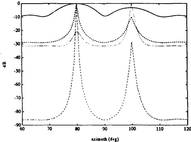
Figure 1: Bispectral DF on Two Sources — Gaussian source at  $80^\circ$  azimuth; bilinear source at  $100^\circ$  azimuth; Gaussian sensor noise. The solid line is the classical DF, the dashed line is MUSIC, the dotted line is bispectral MUSIC, and the dash-dot line is mixed bispectral MUSIC.
