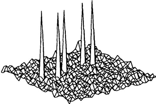
Figure 3: Gabor Transform of the Time Series of the First Sensor — The 11-Hertz signal at 1/10 amplitude, additive  $\mathcal{N}(0,1)$  noise, and the five Gabor transients.
