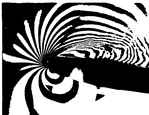
Figure 10(continued). Point Diffraction Interferograms Showing Effect of Frequency on Dynamic Stall Development at Four Angles of Attack. M_\infty = 0.30
