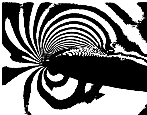
Figure 10(continued). Point Diffraction Interferograms Showing Effect of Frequency on Dynamic Stall Development at Four Angles of Attack. M_\infty = 0.30
