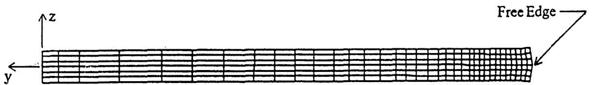
b. Deformed Finite Element Mesh under 100 psi Axial Stress.
