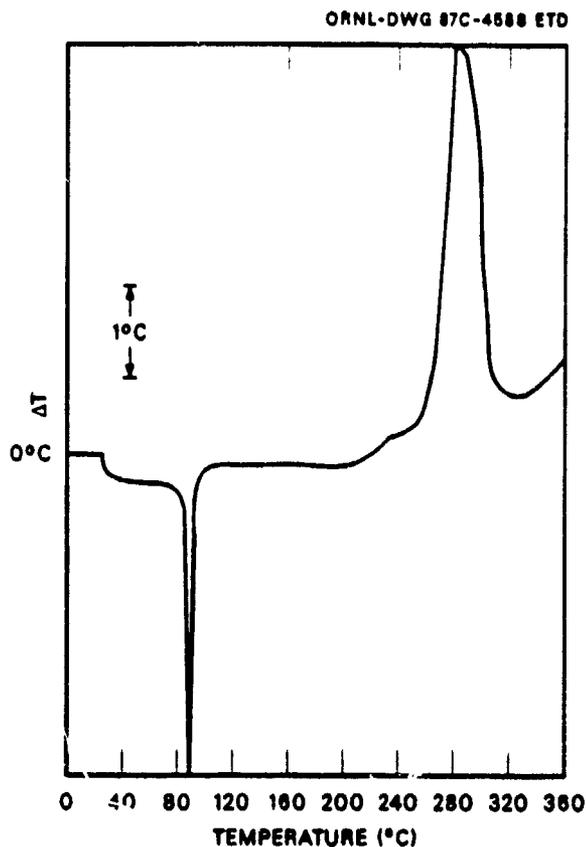
Fig. C.1. DTA curve of recrystallized TNT - melting point 81°C.
