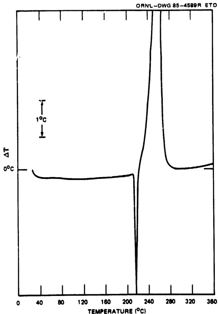
Fig. C.2. DTA curve of RDX (Holston Lot 3-68, 6-441, type A, class E, 99.8%) - melting point indicated at 211°C. Sources: S. W. Dudiel and J. Baytos, *Differential Thermal Analysis Unit*, LAMS-2988, Los Alamos Natl. Lab., Los Alamos, N.M., December 1963, Fig. 20, p. 53.
