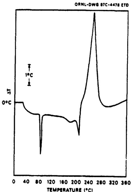
Fig. C.3. DTA curve of Comp. B-3 cast explosive. *Source:* S. W. Dudiel and J. Baytos, *Differential Thermal Analysis Unit*, LAMS-2988, Los Alamos Natl. Lab., Los Alamos, N.M., December 1963, Fig. 24, p. 57.
