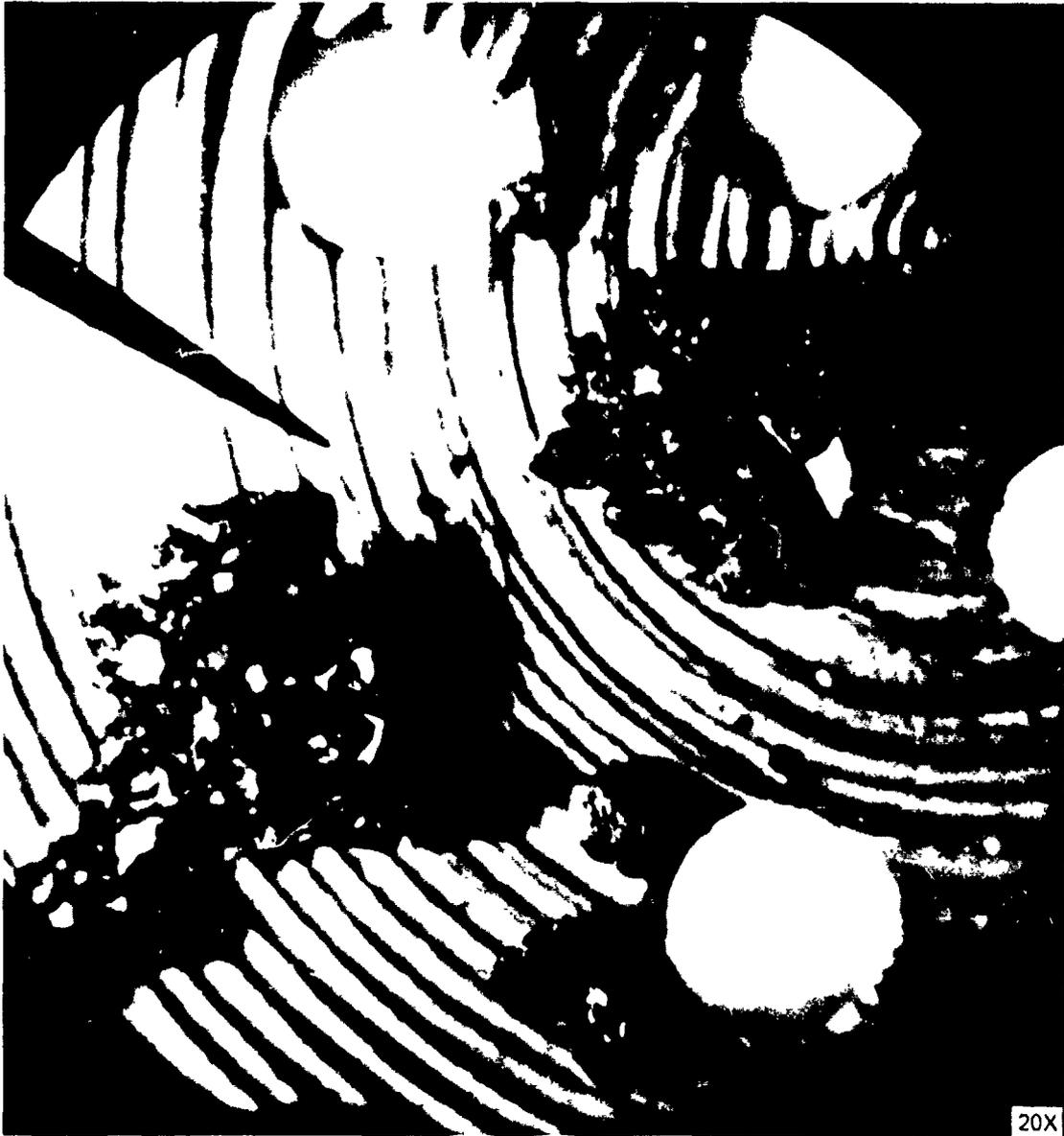
Fig. B.7. Nozzle plate No. 4 [ $\sim 737\text{-}\mu\text{m}$  (0.029-in.) hole size] plugged with 250- by 300- $\mu\text{m}$  particles.
