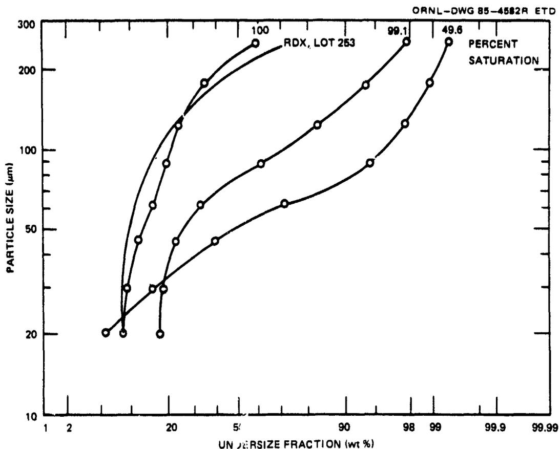
Fig. A.1. Particle-size distribution of RDX (Lot 253) generated by evaporation of acetone in the presence of No. 2 fuel oil.
