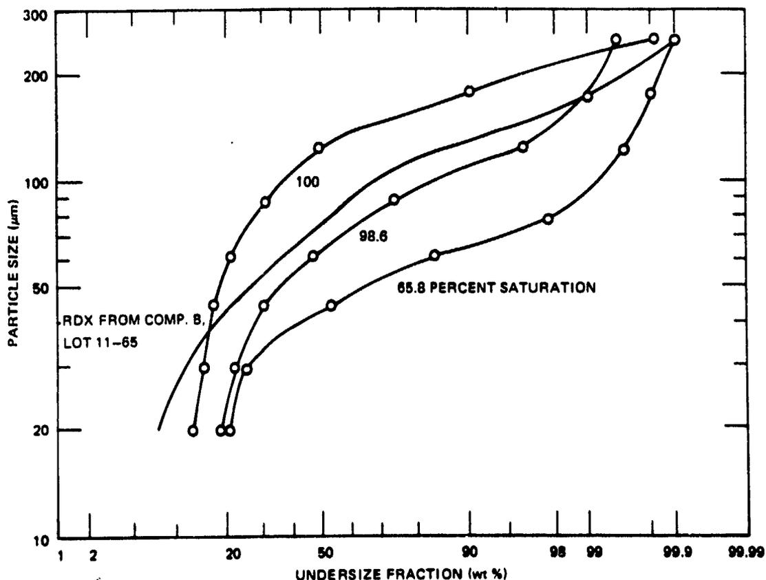
Fig. A.4. Particle-size distribution of RDX (Comp. B, Lot 11-65) generated by evaporation of a mixture of acetone and water (90 : 10) by volume in the presence of No. 5 fuel oil.
