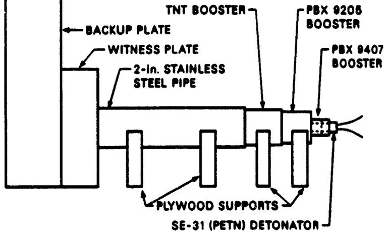
Fig. D.2. Setup for static mode.
