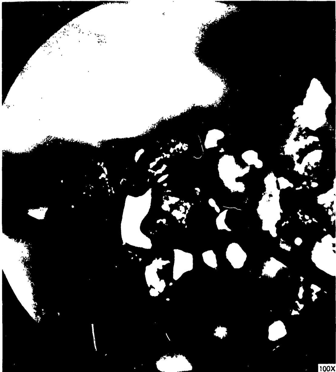
Fig. B.8. Nozzle plate No. 4 [ $\sim 737\text{-}\mu\text{m}$  (0.029-in.) hole size] plugged with 250- by 300- $\mu\text{m}$  particles.
