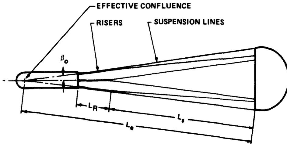
FIGURE 2. EFFECTIVE RIGGING LENGTH WITH MULTIPLE RISER ATTACHMENTS
