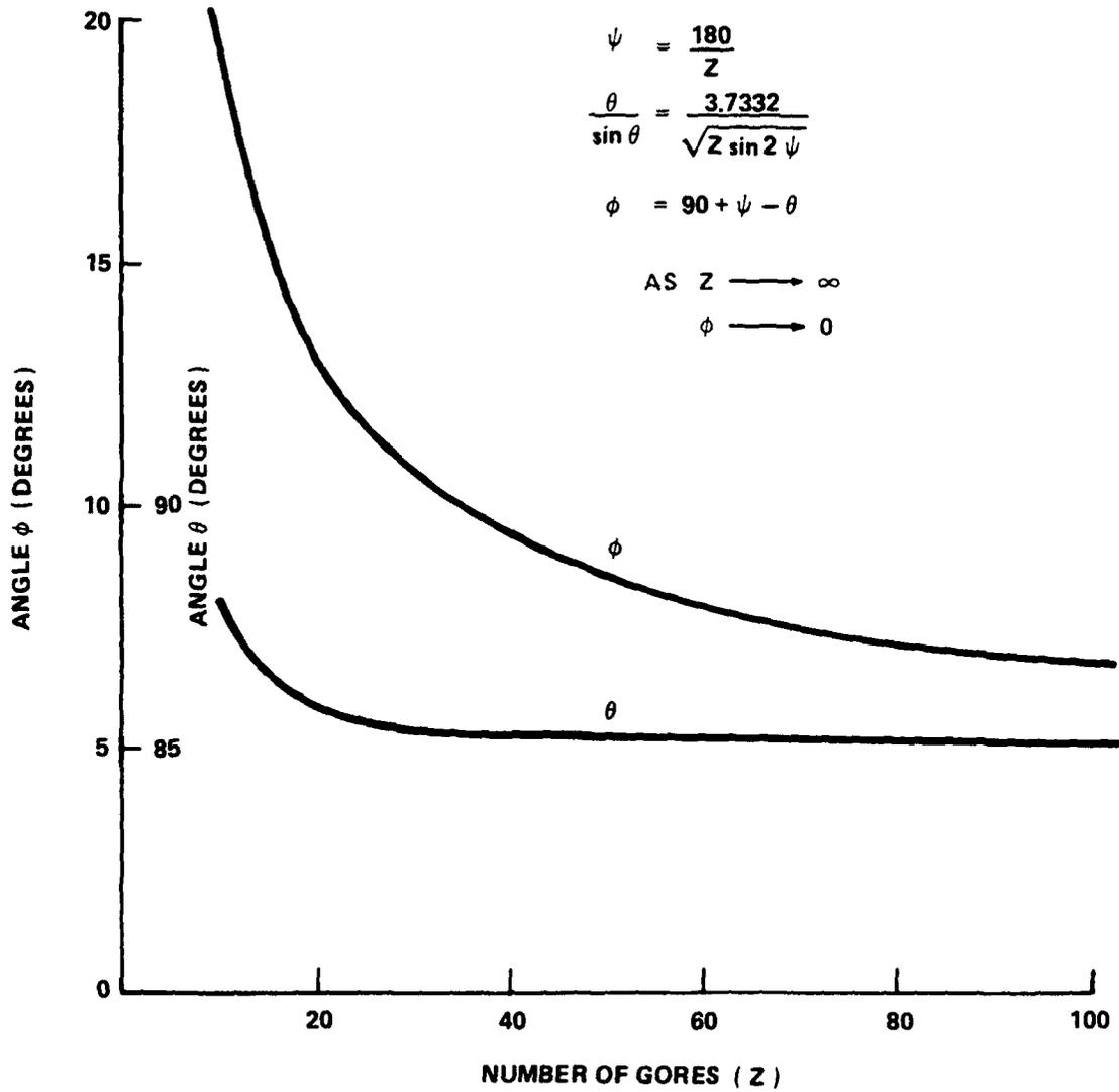
FIGURE 6. EFFECTS OF THE NUMBER OF CANOPY GORES ON THE CLOTH TANGENT FORCE ANGLE  $\phi$  AND GORE BILLOW HALF ANGLE  $\theta$
