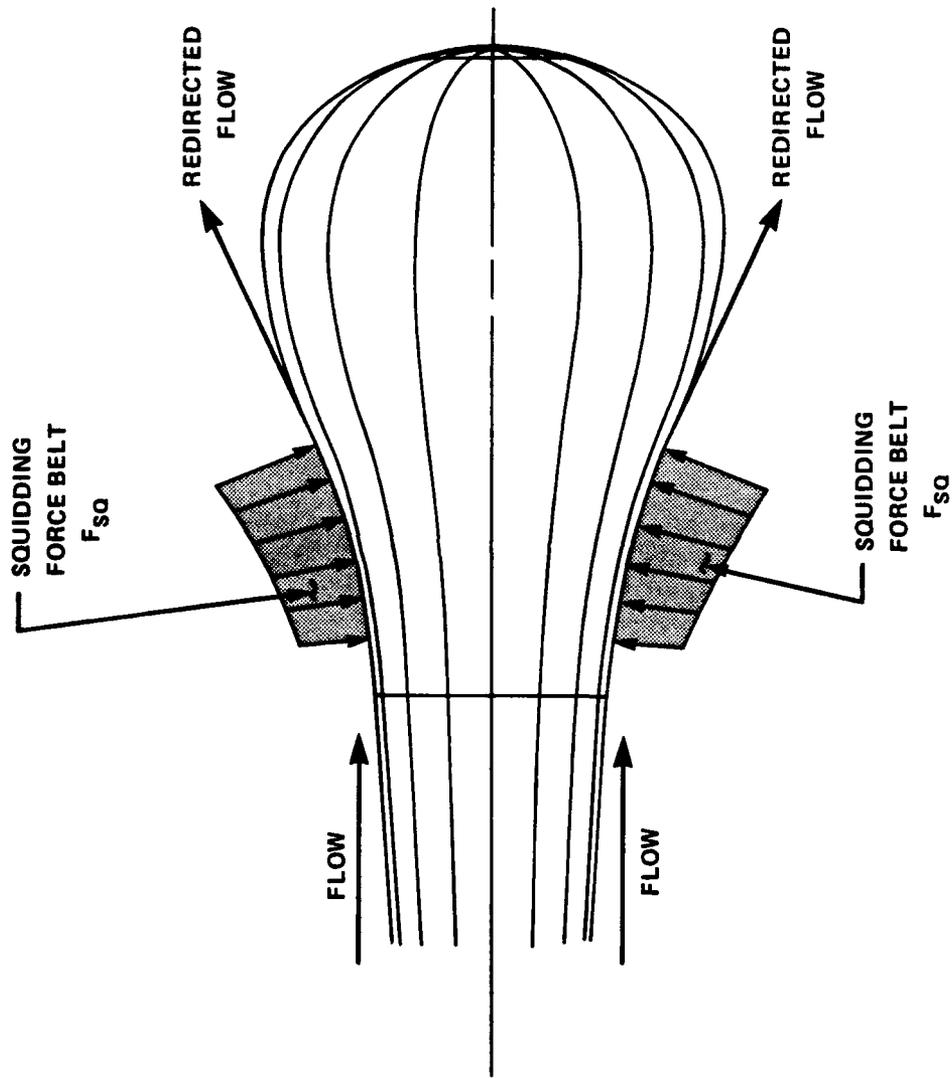
**FIGURE 16. THE REDIRECTED FLOW AROUND A SQUIDDED OR INFLATING PARACHUTE DEVELOPS A SQUIDDING FORCE BELT WHICH STABILIZES THE ASSEMBLY AND MAINTAINS THE SQUIDDED CONDITION BELOW THE UPPER CRITICAL VELOCITY**
