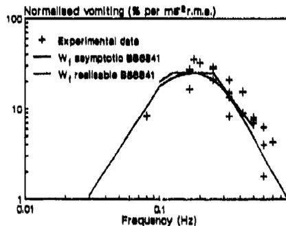
Figure 13 'Normalised vomiting incidence' for 2 h exposures & weighting  $W_v$  from British Standard 6841 (1987). (Data from McCauley et al 1976; normalised vomiting incidence = (% vomiting)/(r.m.s. acceleration,  $\text{ms}^{-2}$ )
