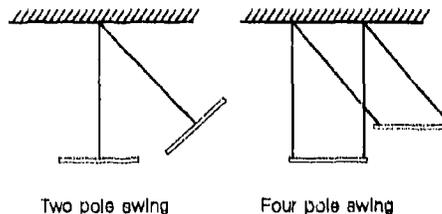
Figure 11 Diagrammatic illustration of 2-pole and 4-pole swings.
