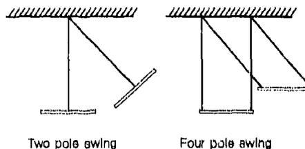
Figure 11 Diagrammatic illustration of 2-pole and 4-pole swings.
