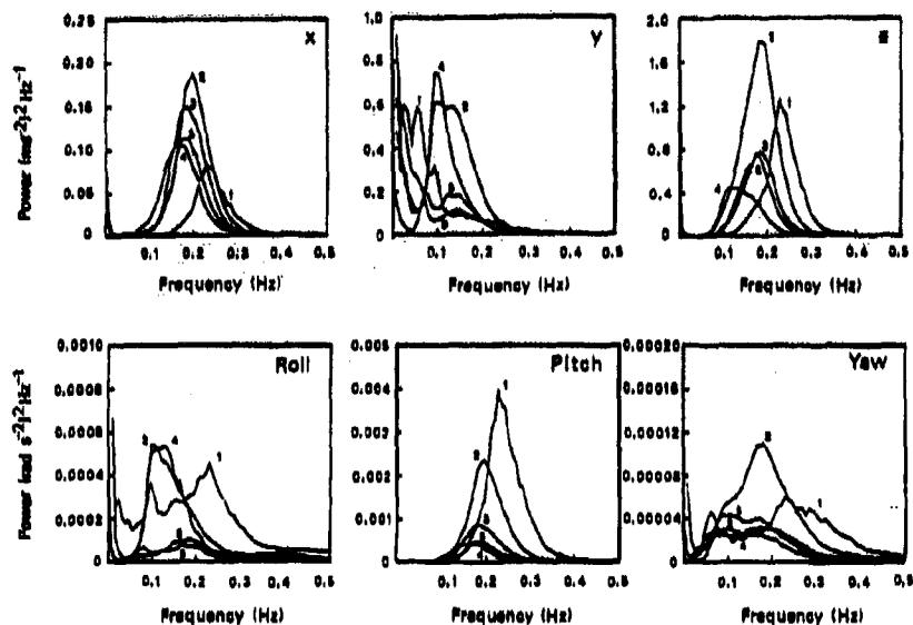
Figure 8 Averaged acceleration power spectral density functions for various voyages on five passenger vessels as reported by Lawther and Griffin, 1988. [Vessel 1: 67 metres; vessel 2: 99 metres; vessel 3: 109 metres; vessel 4: 121 metres; vessel 5: 130 metres. Accelerations apply to the centre of each vessel and are relative to ship-referenced coordinate systems. Frequency resolution 0.01 Hz.]
