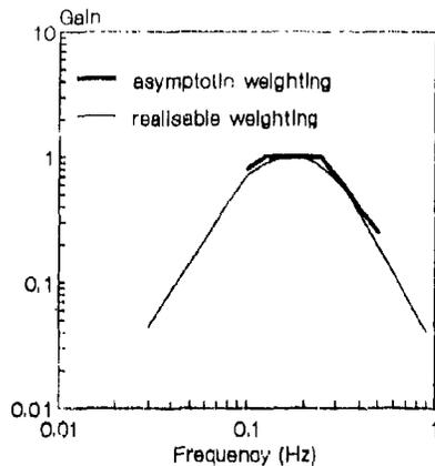
**Figure 9** Frequency weighting  $W$ , as defined in British Standard 6841 (1987). (Graph shows straight line 'asymptotic approximations' to the illustrated realisable weighting defined by the standard for use in instrumentation).
