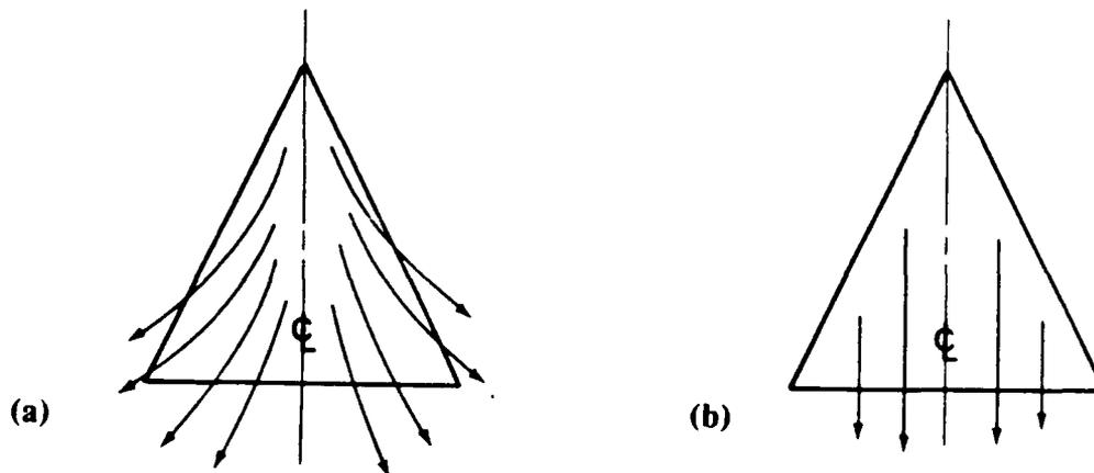
Figure 4.1. Flat Bottom, Delta Wing Configuration (b) versus Waverider Streamlines (a) (9:400)
