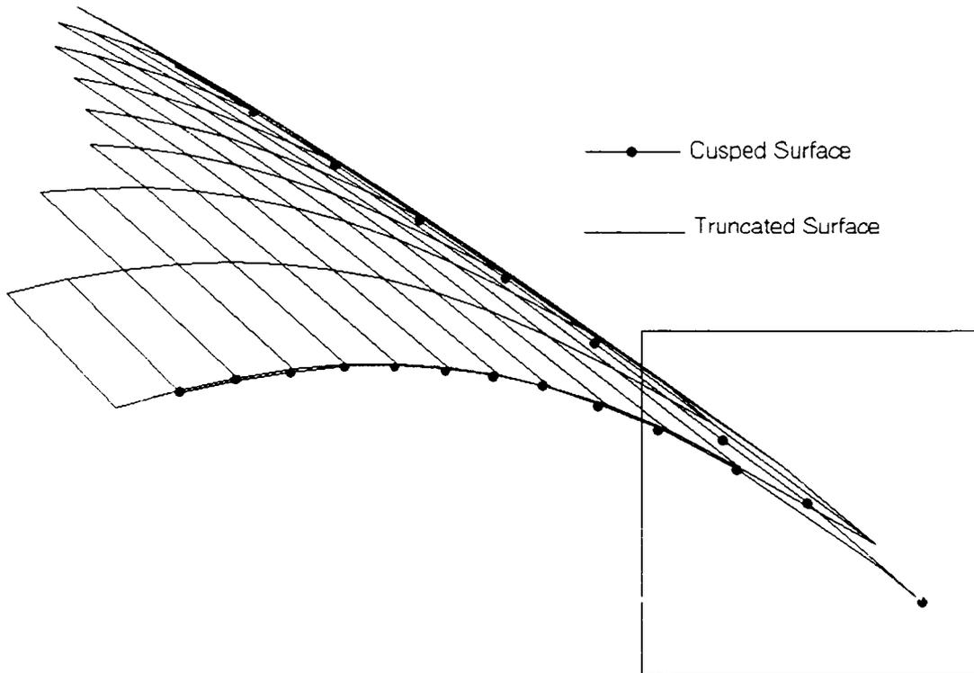
**Figure 2.6.** Cusped and Truncated Leading Edge Design
