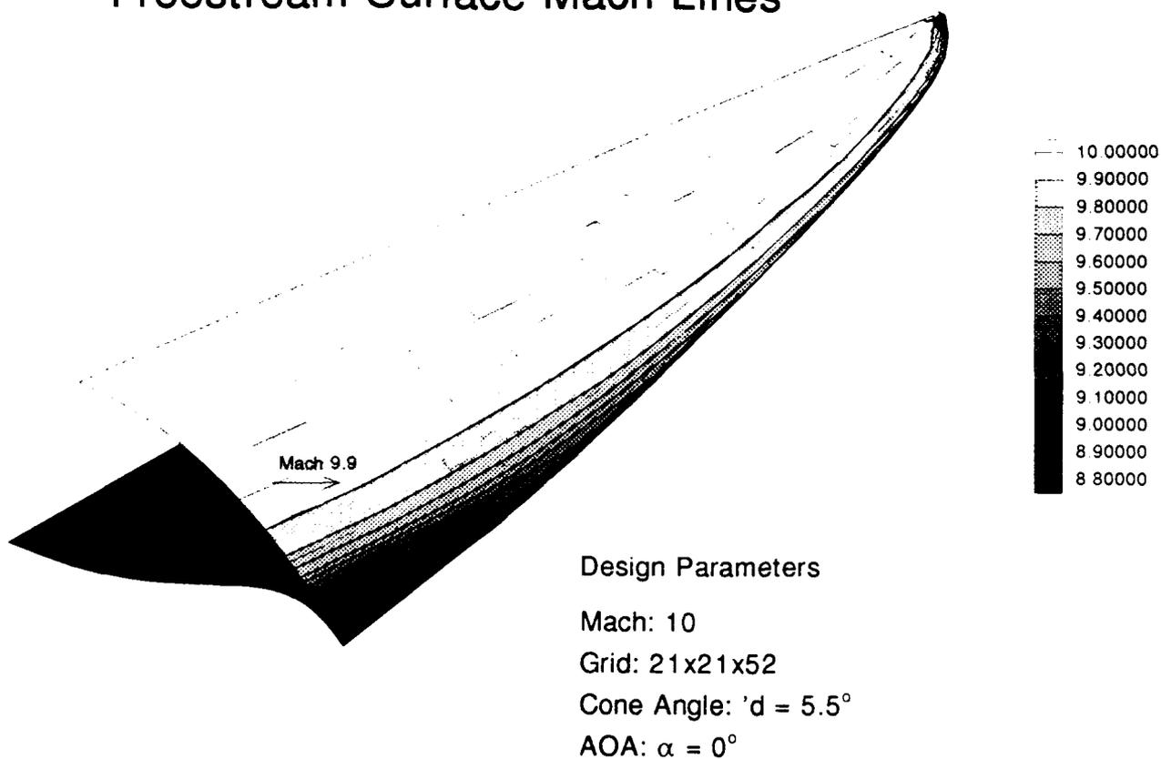
Figure 5.2. Flow Expansion to the Freestream Surface
