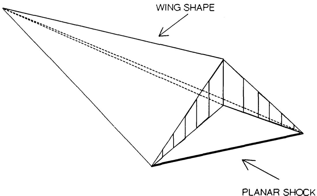
**Figure 1.2.** Caret Wing Planar Waverider
