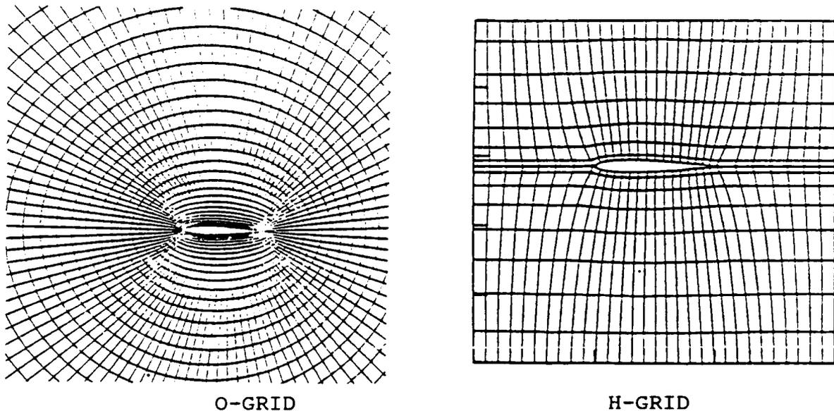
**Figure 2.3.** O-grid and H-grid Implementation
