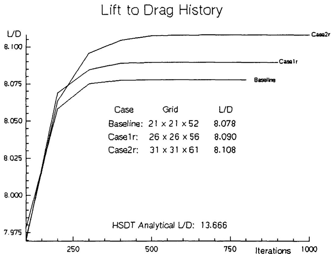
**Figure 4.14.** L/D History versus Grid Refinement
