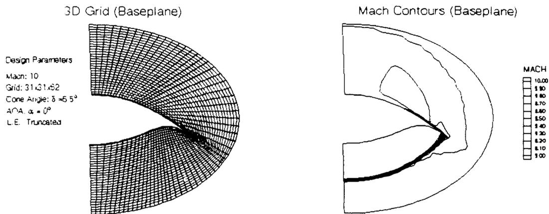
**Figure 4.15.** Conical Shock Wave Refinement: Case 1r
