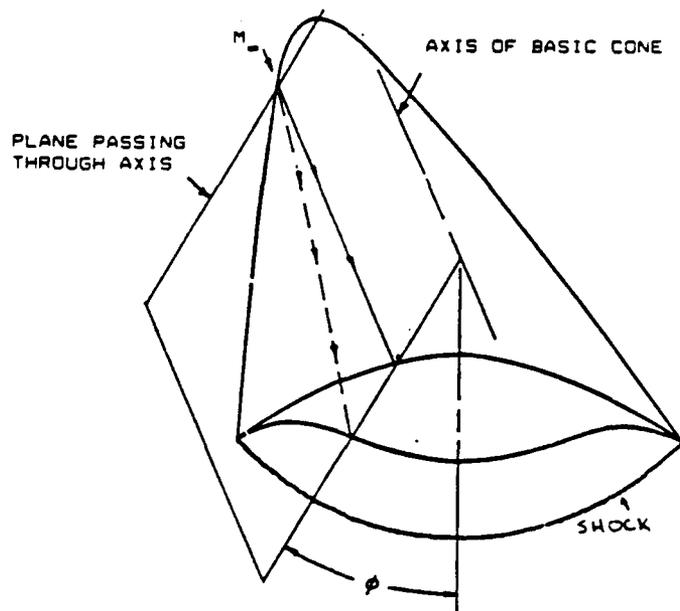
**Figure 1.5.** Waverider Design Methodology (16:7)
