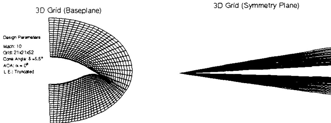
Figure 4.2. Grid Structure: Baseline ( 21 x 21 x 52 )
