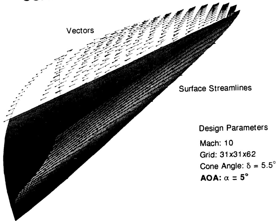
Figure 4.22. Compression Surface Streamlines:  $\alpha = 5^\circ$
