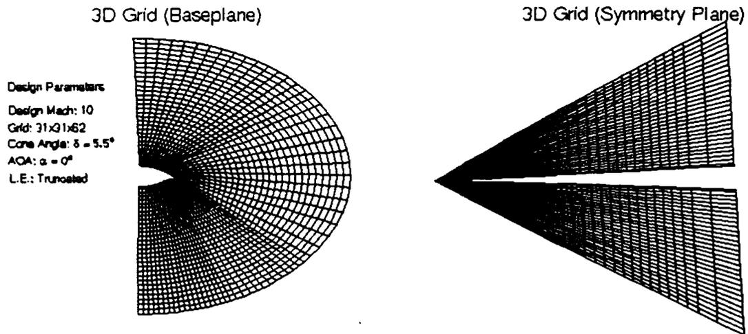
**Figure 4.16.** Grid Structure: Expanded Domain (31 x 31 x 62)
