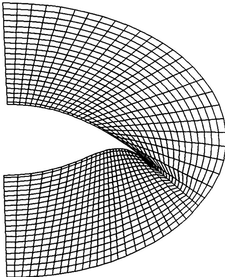
Figure 4.8. Grid Structure: Cusped ( 21 x 21 x 52 )
