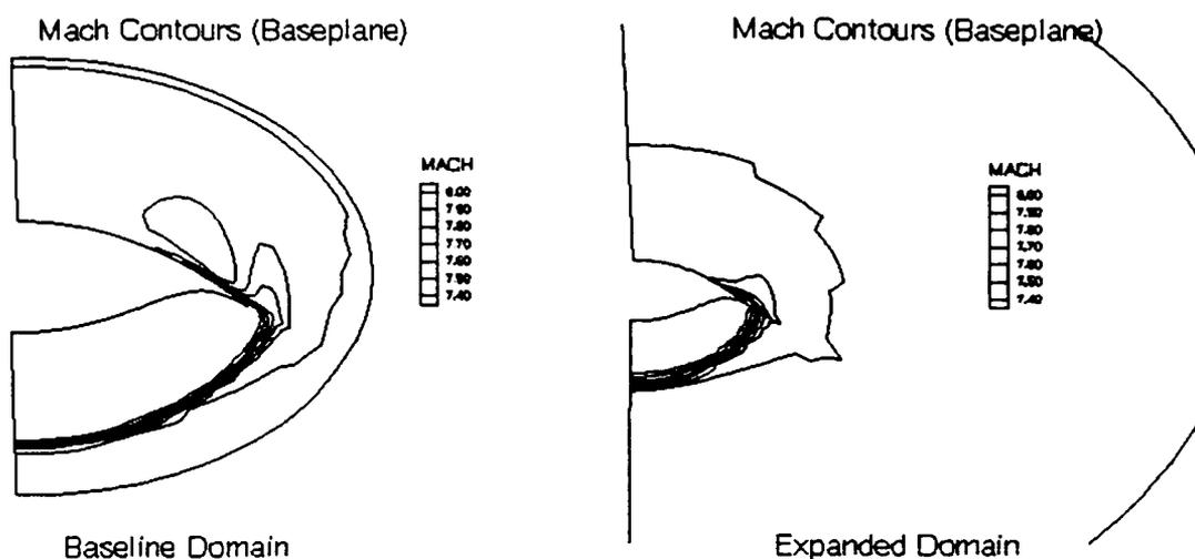
**Figure 4.17.** Conical Shock Wave Development: Mach 8.0
