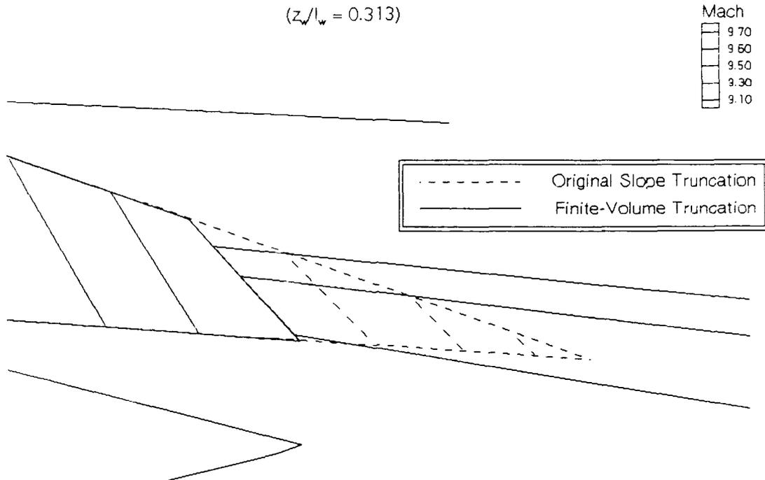
**Figure 4.10.** Numerical Truncation: Cell-Centered Approximation
