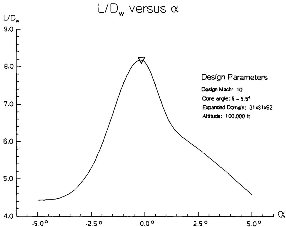
**Figure 4.23.** L/D versus Angle of Attack
