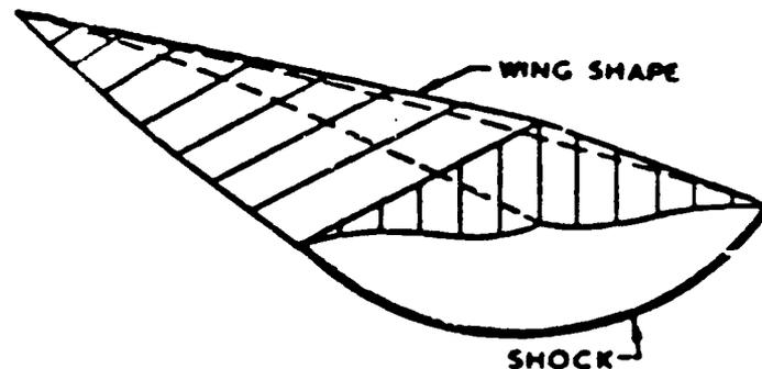
**Figure 1.1.** Waverider With Attached Shock Wave (3:12)
