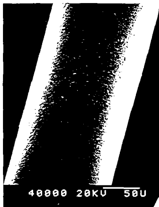
Photo.2 SEM of Ni Coated Fiber (400 X)
