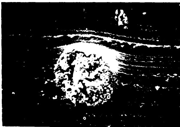
Figure 7. Clay Agglomerates in Defective Filled Polyethylene Insulation
