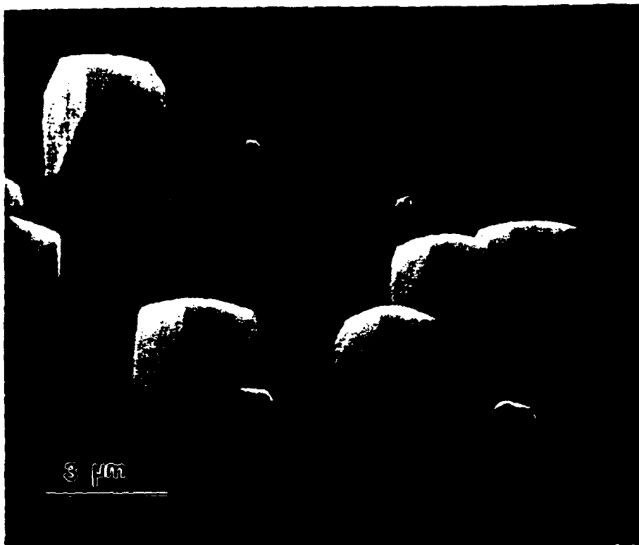
Figure 4. SEM of center region taken at 45 deg. tilt to show (111) faceting.
