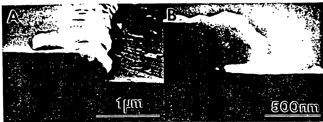
Figure 6. Cleaved cross-section showing ELO of diamond over a Si mask that has been chemically removed: (A) inclined view and (B) edge-on view.
