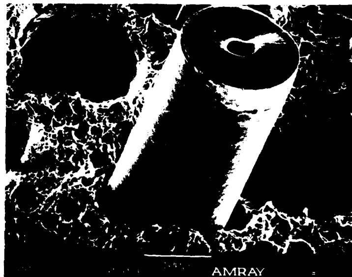
Figure 48. Fracture surface of notched [0^\circ]_8 specimen away from hole.
