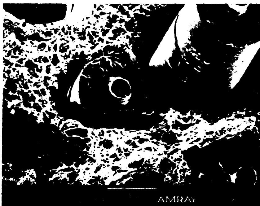
Figure 46. Fracture surface of unnotched [0^\circ]_s specimen.
