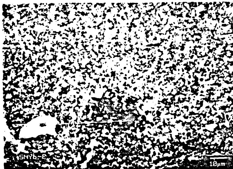
a. A 25 to 30 \mu\text{m} Impurity (Fe) Affected Region. Mag. 800X
