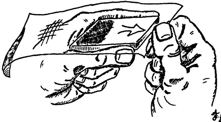
Figure 3.1: The "zero-G" wipe: a lens cleaning tissue is dragged across the substrate in the direction indicated; the solvent spreads across its surface and evaporates before reaching the end of the tissue.
