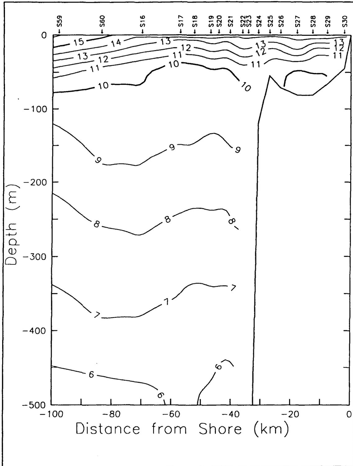
**Figure 5a. Farallones Transection Temperature Field:** Temperatures in °C along the Farallones Transection. CTD station locations are indicated along the top of the figure.
