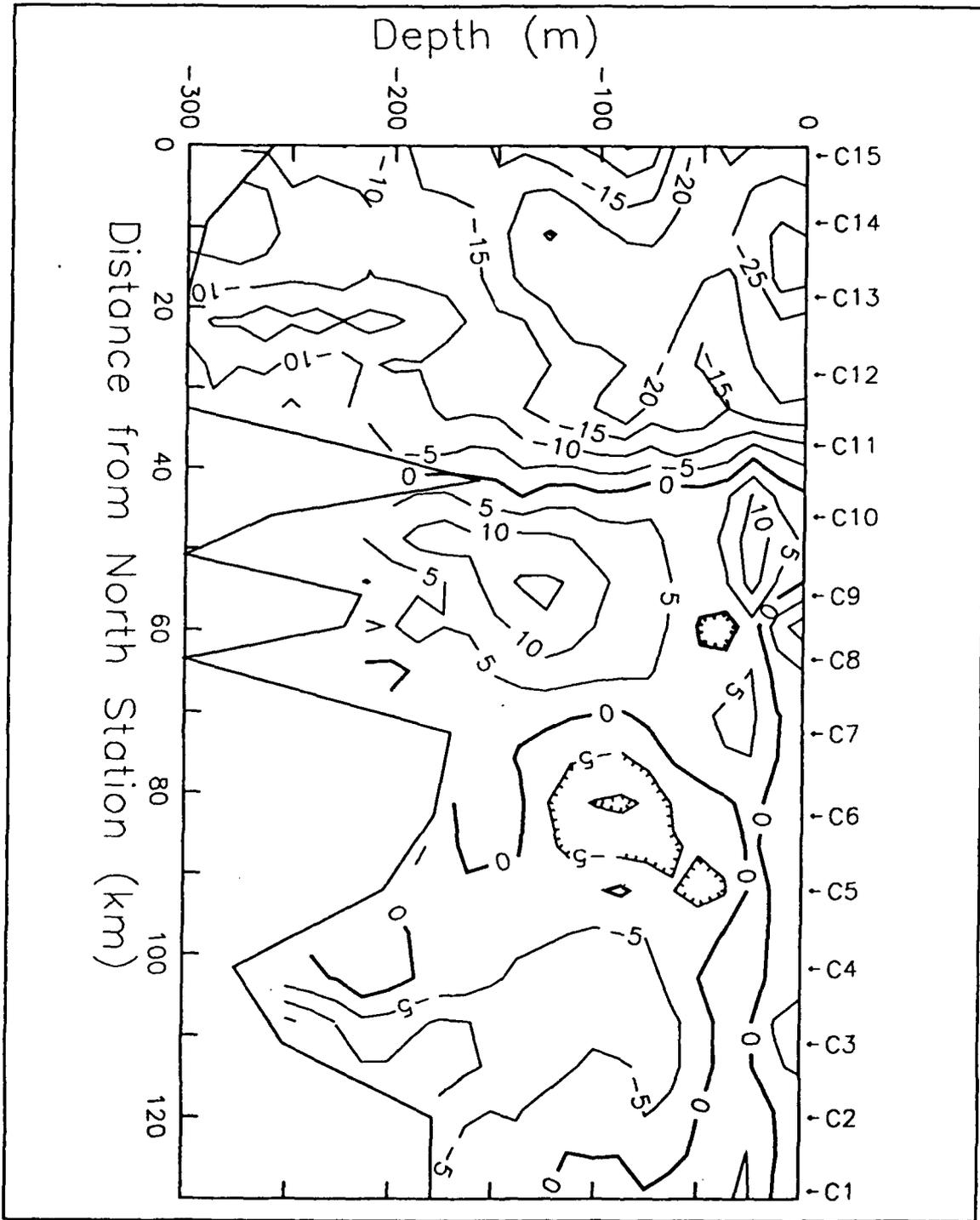
**Figure 4e. Offshore Transection Detided ADCP East-West Velocity:** East-west velocities in cm/s along the Offshore Transection. Positive values indicate eastward velocities. CTD station locations are shown along the top of the figure. Hatching indicates a minimum.
