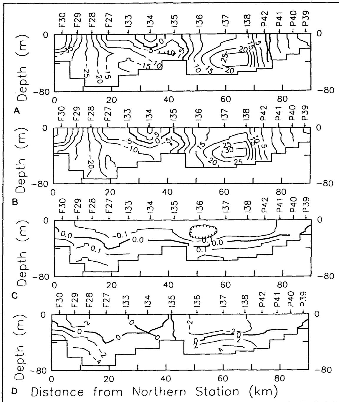
**Figure 10. Salt Flux Quantities Around the Gulf of the Farallones:** (a) Detided cross-transsection velocities in cm/s. Positive values indicate flow into the Gulf. Hatching indicates a minimum. (b) Detided cross-transsection velocity with mean removed in cm/s. (c) Salinity field with mean removed  $S'$  in psu. (d) Salt flux field  $V'_c S'$  in psu-cm/s. Positive values denote flux into the Gulf.
