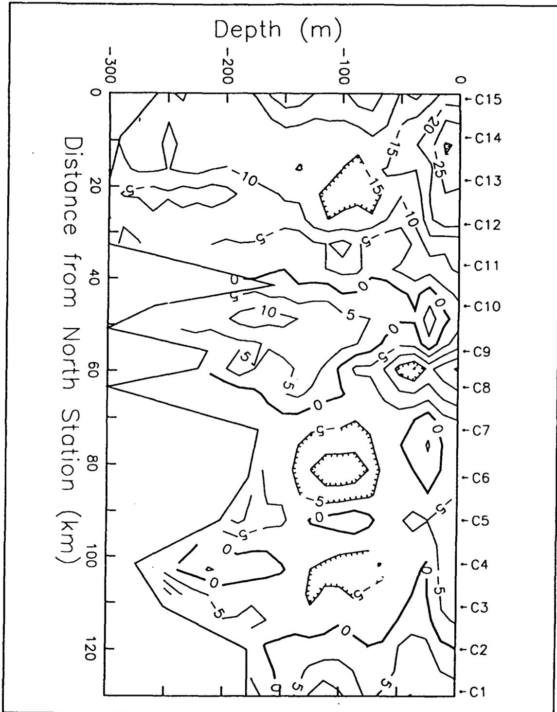
**Figure 4g. Offshore Transection Detided ADCP Cross Velocity:** Cross-transsection velocities in cm/s along the Offshore Transection. CTD station locations are shown across the top of the figure. Hatching indicates a minimum. Positive values indicate flow toward the coast.
