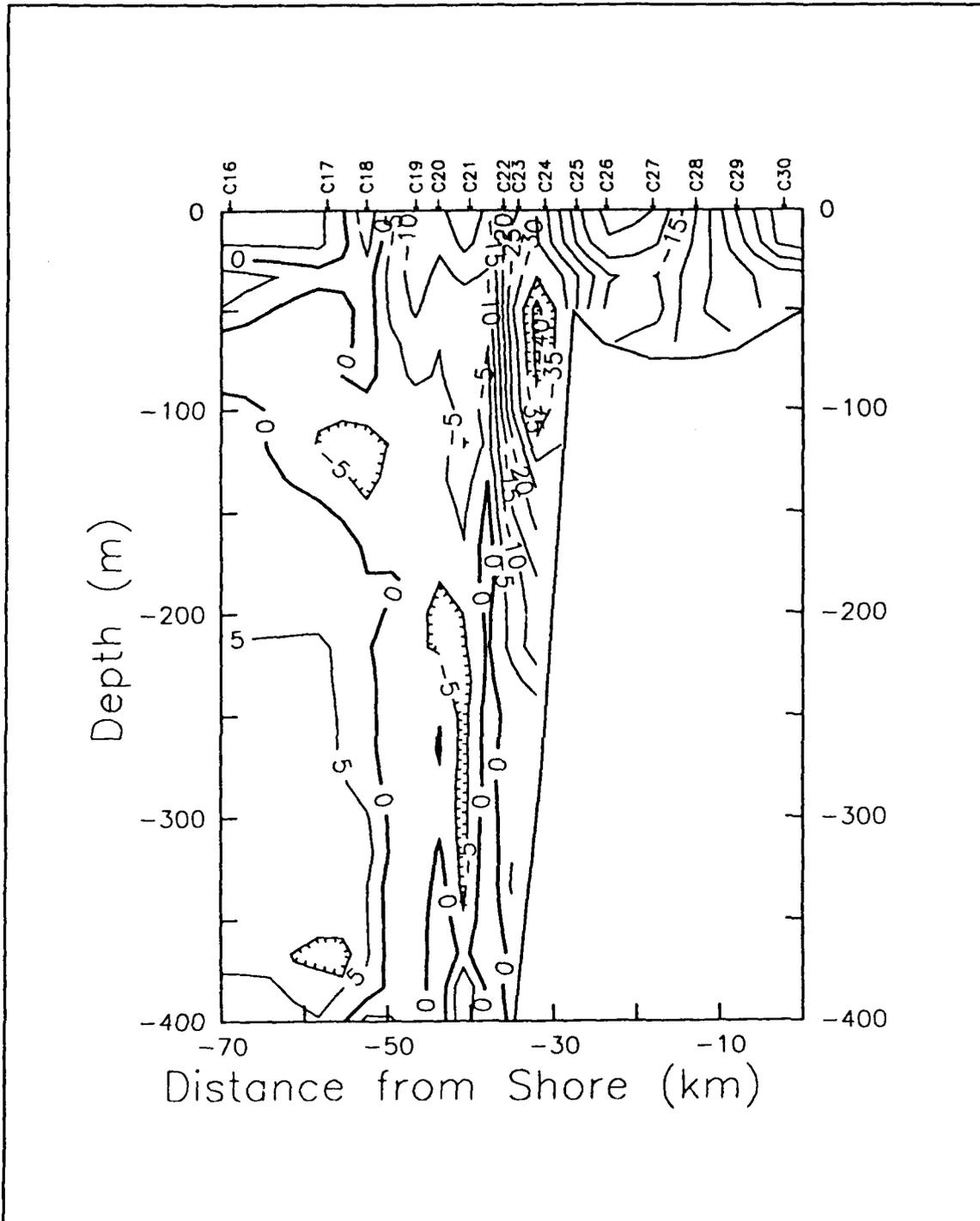
**Figure 5g. Farallones Transection Detided ADCP Cross Velocity:** Cross-transsection velocities in cm/s along the Farallones Transection. Positive values indicate south-eastward flow. CTD station locations are shown along the top of the figure. Hatching indicates a minimum.
