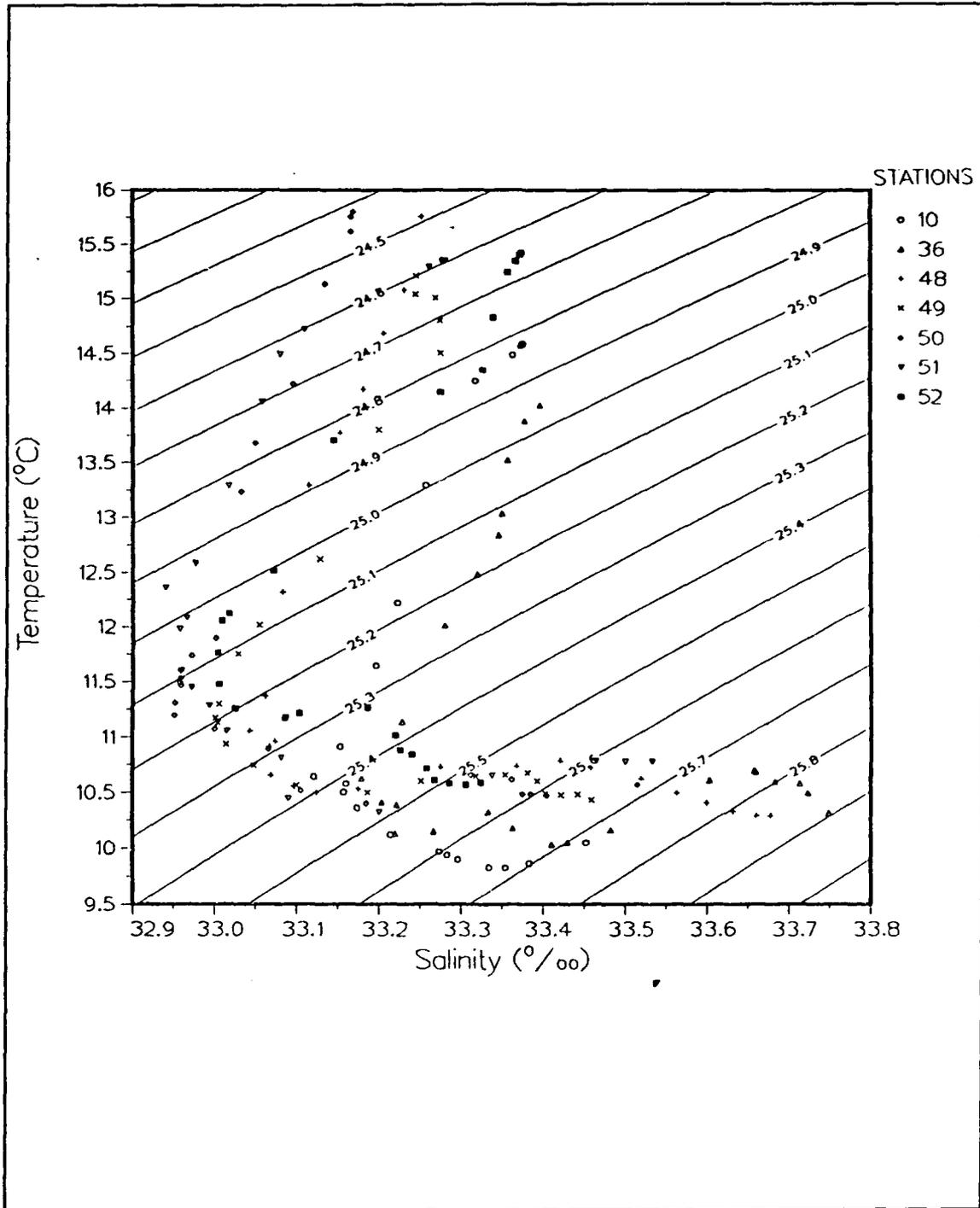
**Figure 8. Temperature and Salinity Properties of Salinity Inversions:** Only stations where the difference between sea surface salinity and the salinity minimum was 0.2 psu or greater are shown. Temperature and salinity values are shown for the upper 50m.
