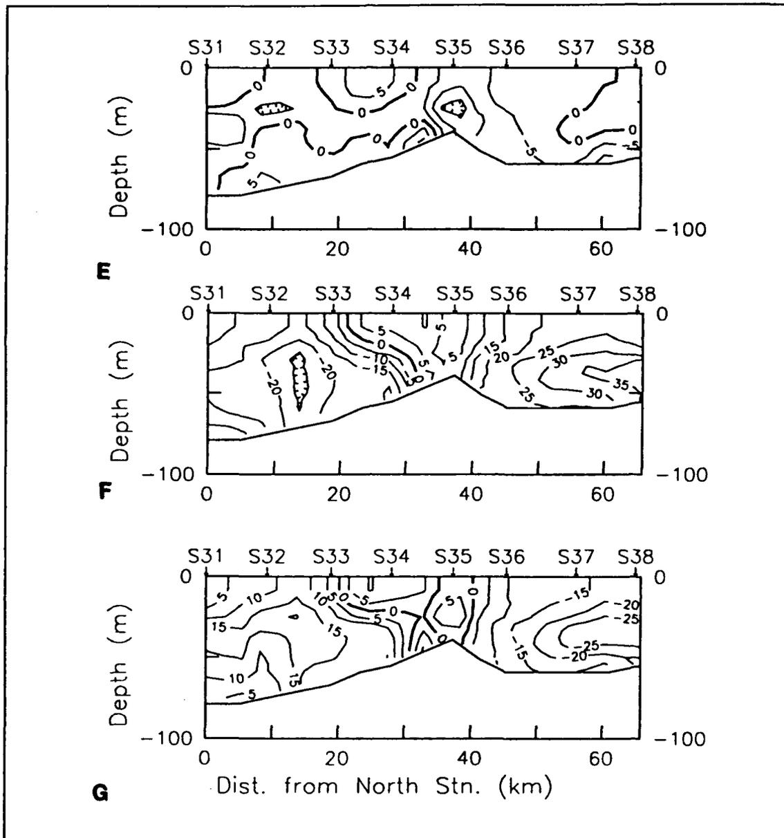
**Figure 3e. Inshore Transection Detided ADCP East-West Velocity:** East-west velocities in cm/s, along Inshore Transection. Positive values indicate eastward velocities. CTD Station locations are shown along the top of the figure. Hatching indicates a local minimum.
