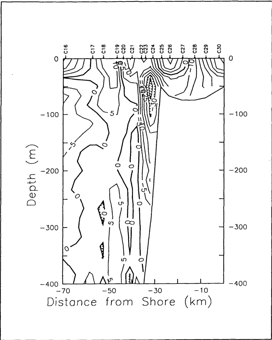
**Figure 5e. Farallones Transection Detided ADCP East-West Velocity:** East-west velocities in cm/s along the Farallones Transection. Positive values indicate eastward velocities. CTD station locations are shown along the top of the figure. Hatching indicates a minimum.
