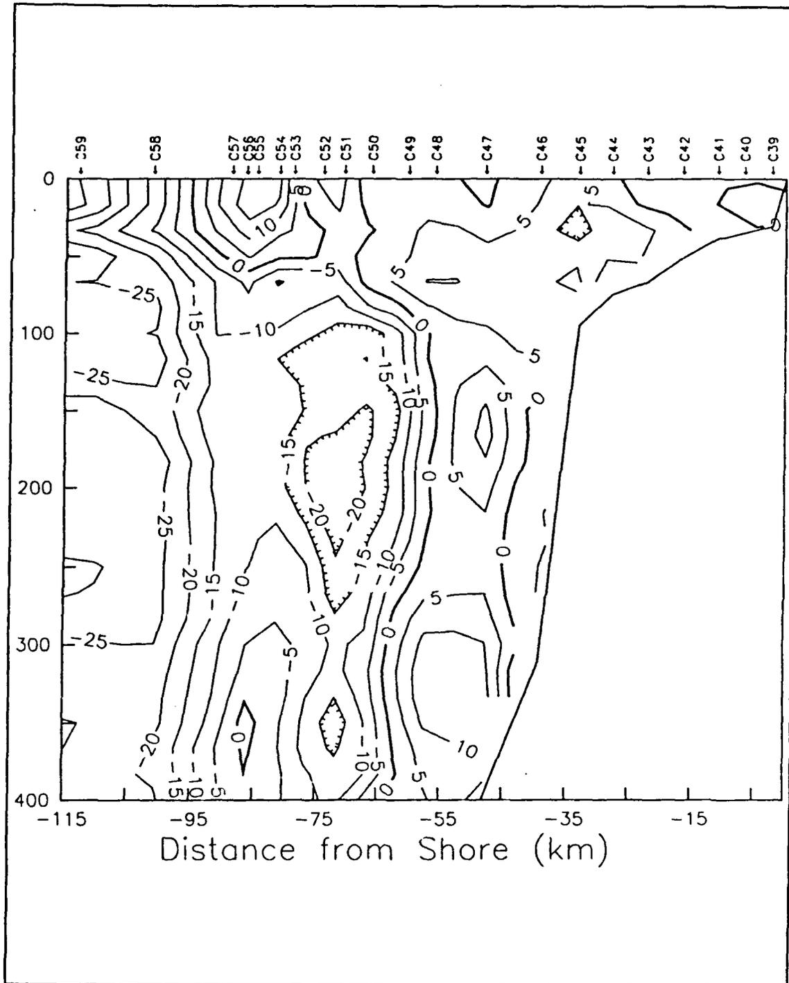
**Figure 6e. Pioneer Transection Detided ADCP East-West Velocity:** East-west velocity in cm/s along the Pioneer Transection. Positive values indicate eastward velocities. CTD station locations are indicated along the top of the figure. Hatching indicates a minimum.
