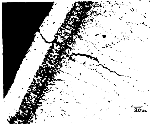
Figure 17: Carbide stain used to delineate structure without etching. The micrograph reveals a fatigue crack running down a substrate grain boundary.
