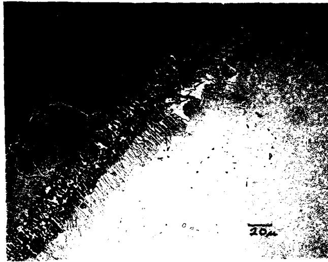
Figure 4: Optical micrograph showing the effect of etchant (1) on the substrate and coating. The coating grain structure is revealed (showing less precipitates than fig. 3 due to solutioning during service) and the substrate \gamma , \gamma' , carbides and grain boundaries are clearly seen.
