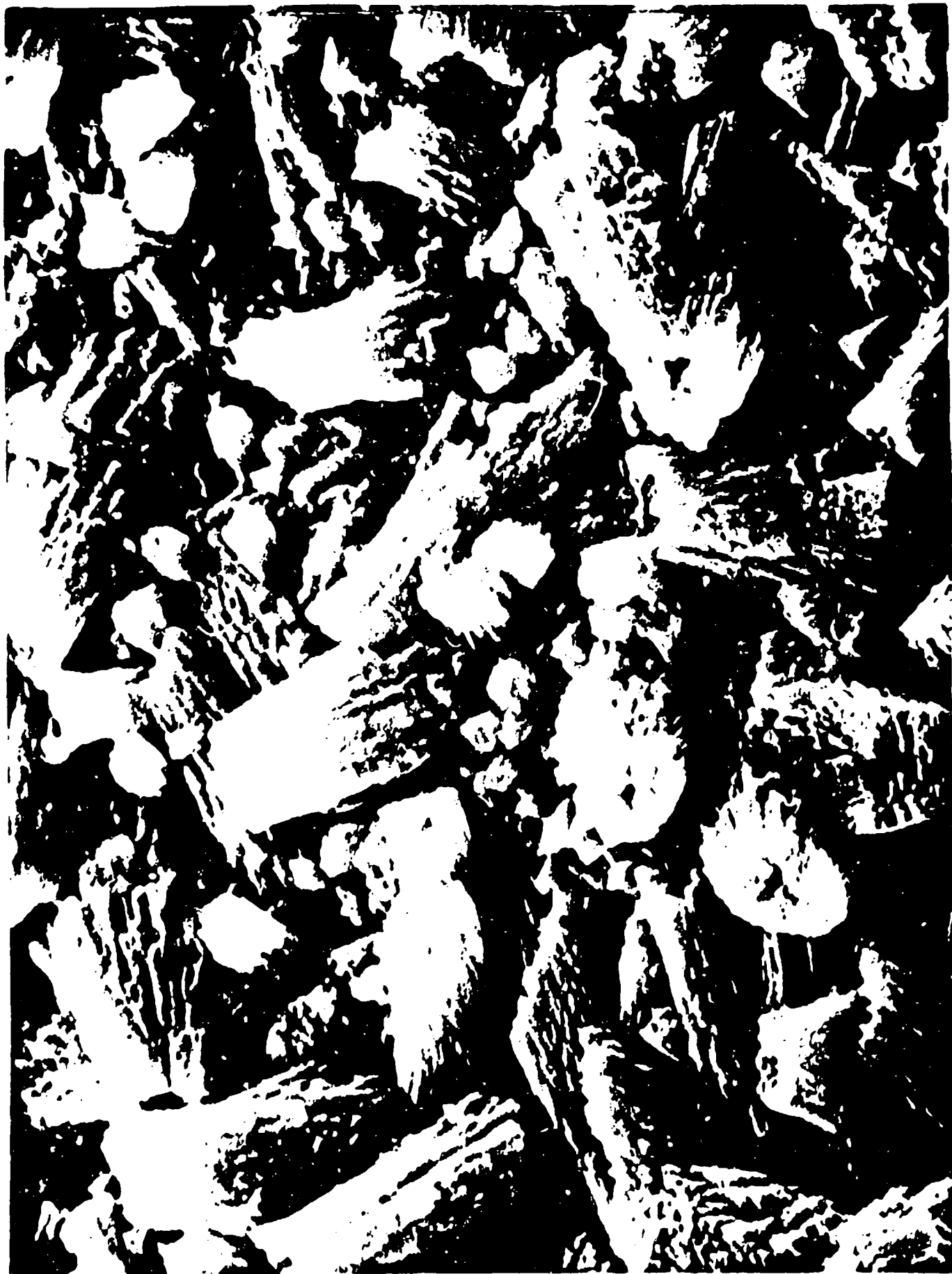
Figure 2. SEM Photograph of AlO_x Surface at 2500X Showing Aluminum Hydroxide Encrustations
