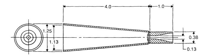
Figure 1. Nozzle Used for Commercial CFC Blend Field Tests 3, 4, and 7.
