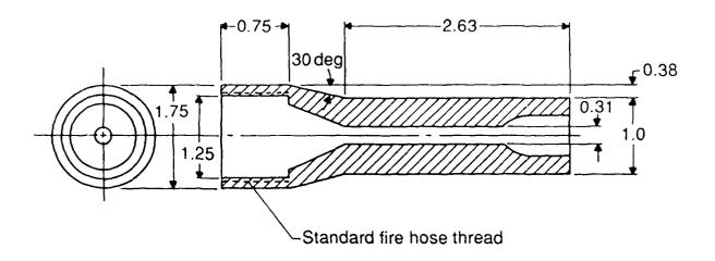
Figure 3. Nozzle Used for Commercial CFC Blend Field Test 11.
