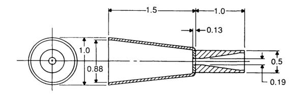
Figure 2. Nozzle Used for Commercial CFC Blend Field Tests 8 and 9.
