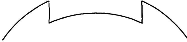
Figure 4: Predicted intensity profile of specularly reflecting concave non-Lambertian radiator
