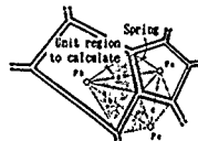
Fig.2 Rigid Body Spring Model with Polygonal shape
