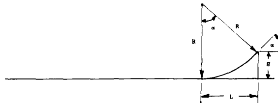
FIGURE A8. RAMP GEOMETRY
