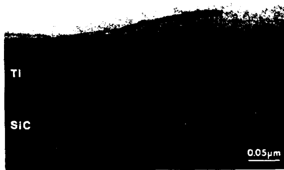
Figure 9. XTEM micrograph of Ti/6H-SiC; Ti deposited at 400°C.
