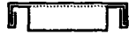
a. Cross section of a single channel containing active material enclosed in a nickel-plated steel envelope.
