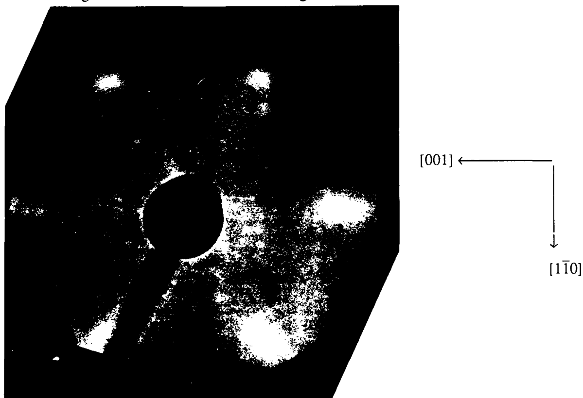
Figure 19. LEED patterns observed on BN deposited on a Cu (110) substrate showing basic (110) pattern (Beam=95.0 V).
