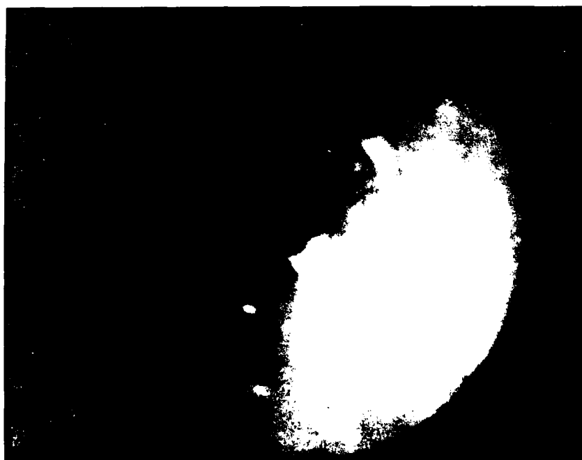
Figure 10b. \beta -SiC RHEED pattern from (110) reflection.
