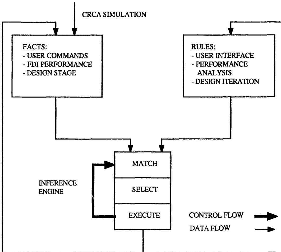
Figure 3-1: FDI Control and Data Flow
