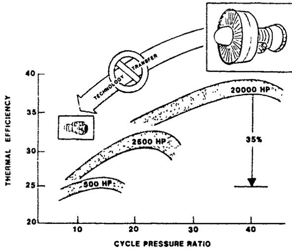
FIGURE 3. - SMALL ENGINES ARE NOT AS EFFICIENT.
