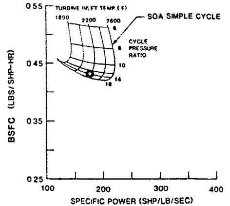
FIGURE 4. - STATE-OF-THE-ART CYCLE PERFORMANCE: 800 HP SLS.
