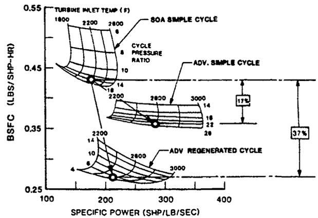
FIGURE 6. - IMPACT OF ADVANCED TECHNOLOGY ON CYCLE PERFORMANCE: 800 HP SLS.
