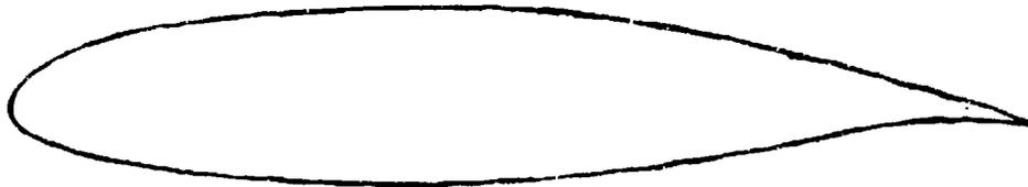
NACA MS(1)-0313      Radius of curvature: 1.5928 % of chord      Thickness: 13% of chord
