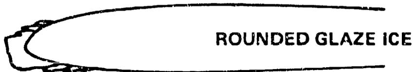
**FIGURE 2-68. HIGH SPEED ICE SHAPES (REFERENCE 2-35)**
