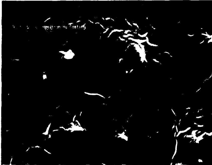
Figure 5: SEM Photograph of Flux at 1000x, Heated at 75°C.
