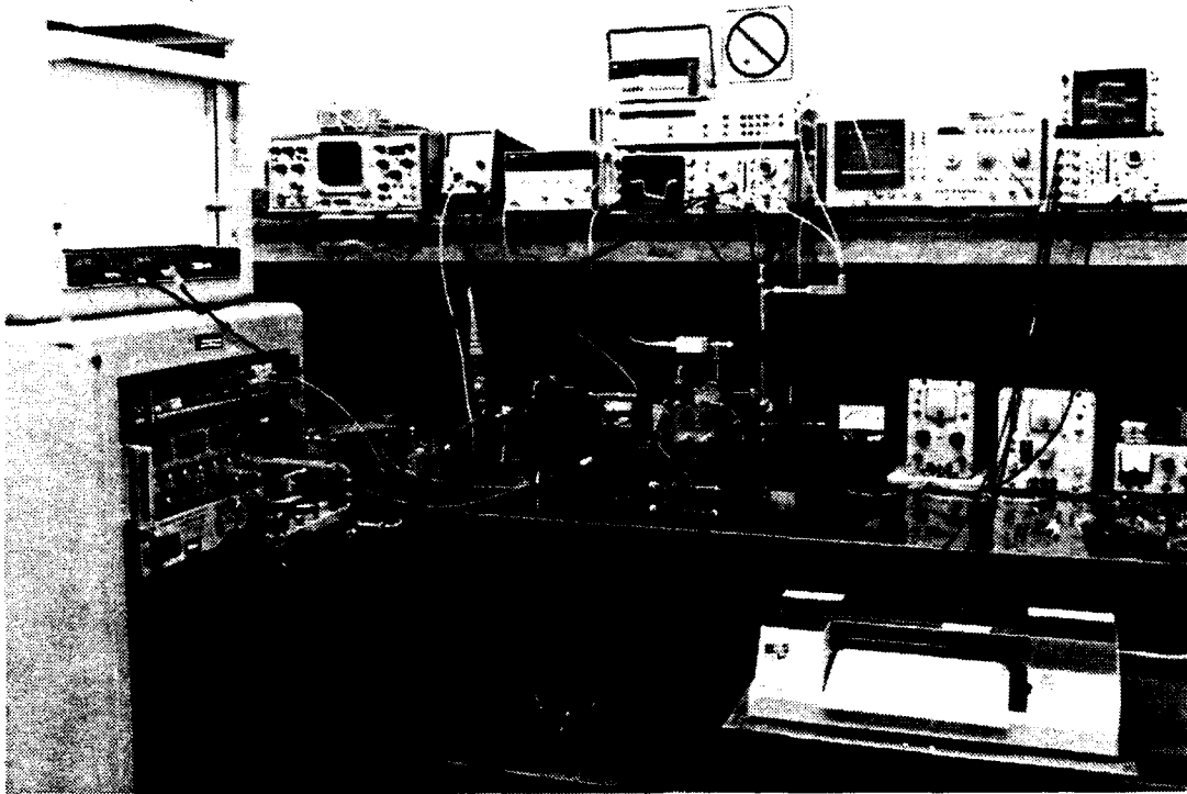
FIGURE 50. Ka-Band Reflectometer System.
