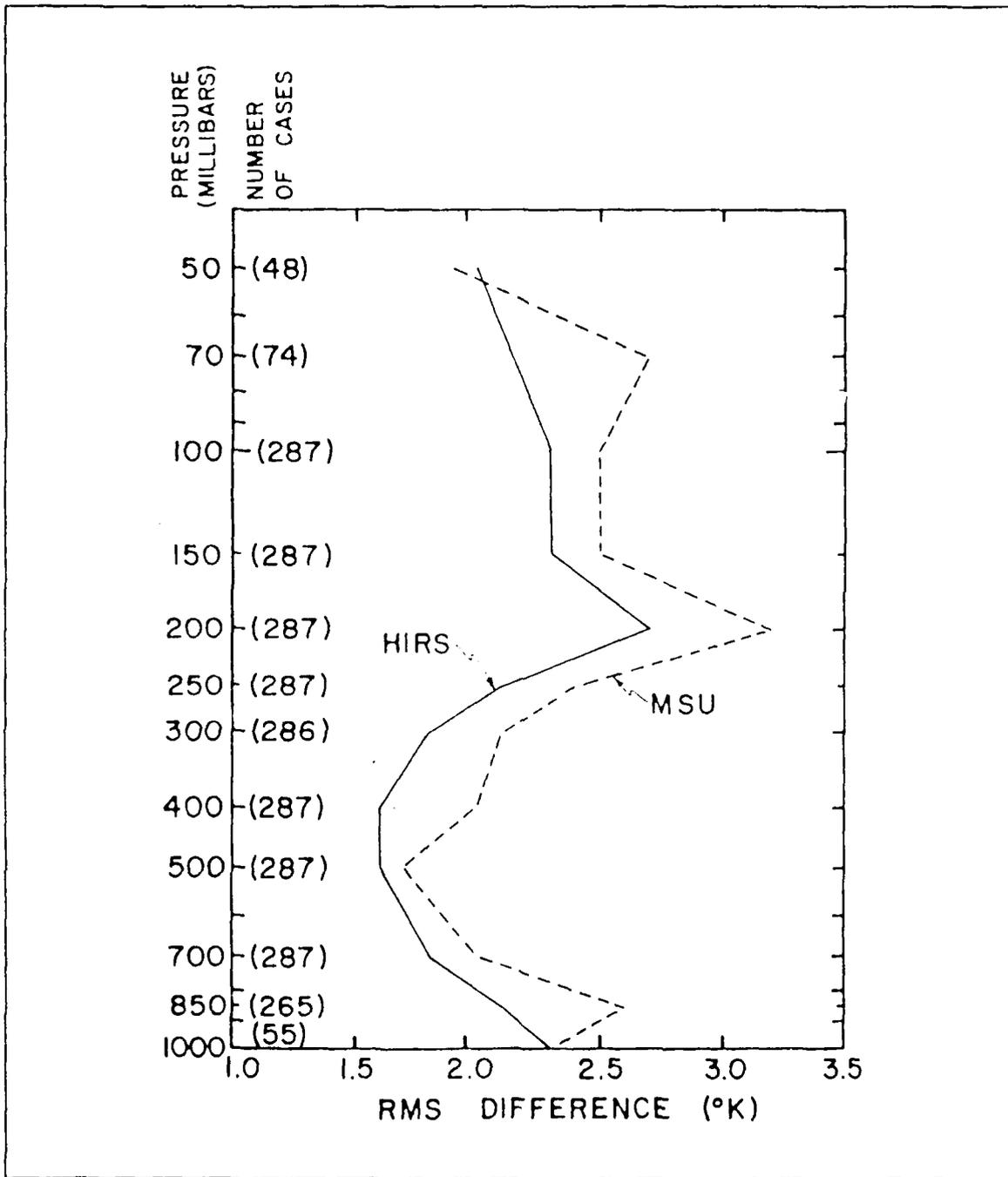
Fig. 3. TOVS and radiosonde composites. The rms difference between North American interactively derived TIROS-N soundings and radiosondes, 22 March-19 April 1979 (From Smith et al. 1979).
