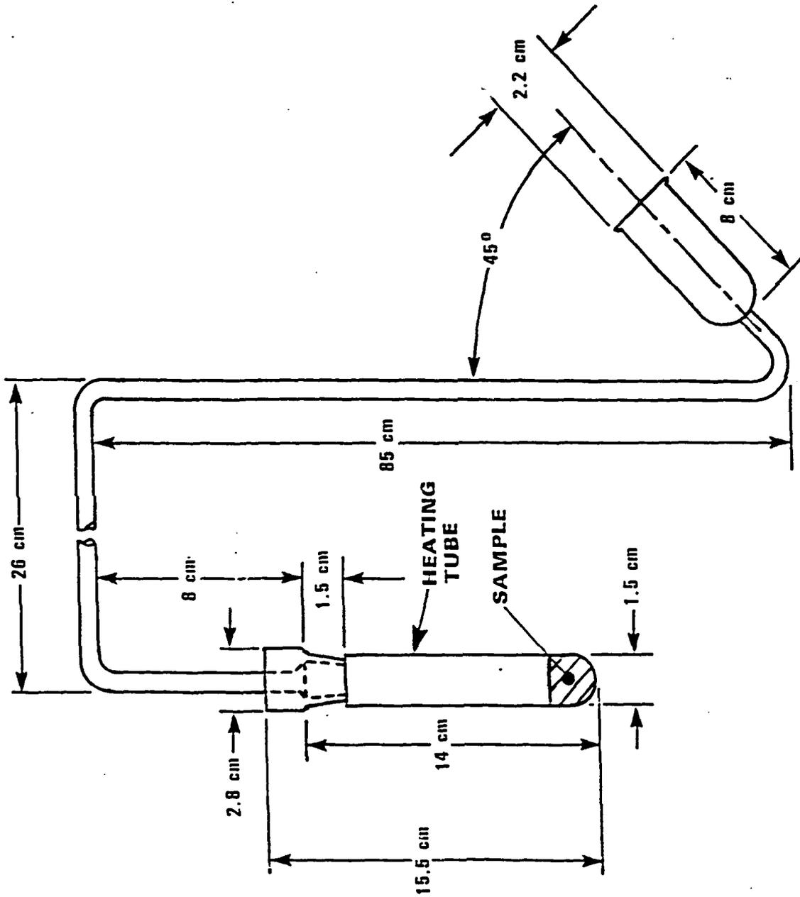
Figure 1. A typical vacuum stability test apparatus
