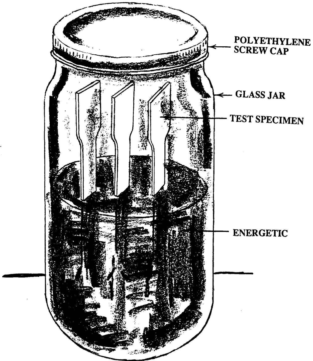
Figure 3. Storage test apparatus
