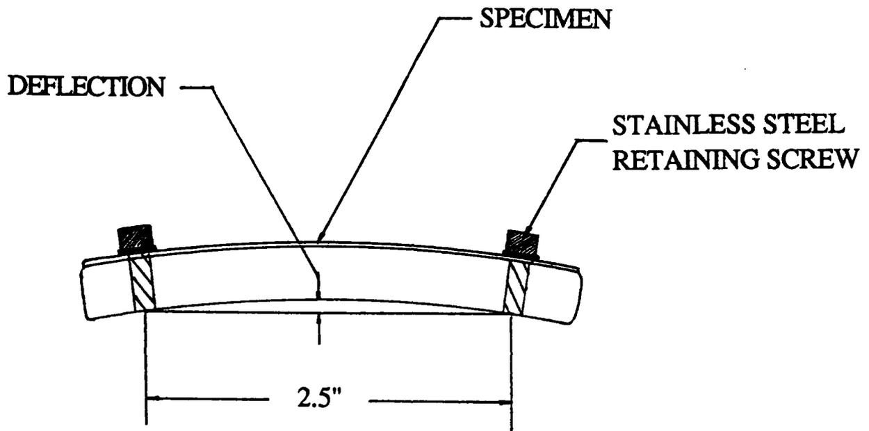
Figure 6. Bending stress fixture.
