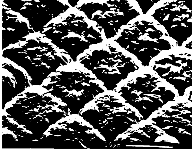
Fig. 3. Surface morphology of diamond film grown on etched Ge.
