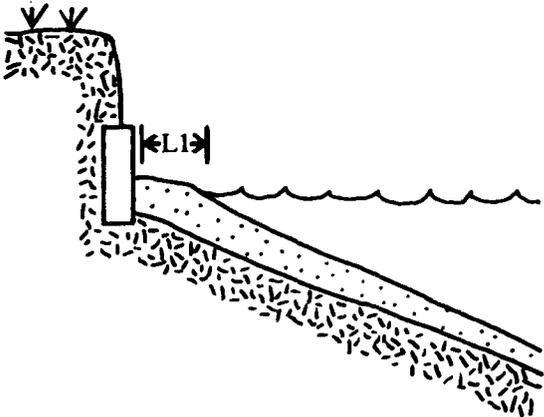
Seawall has approximately the same effect on the beach as would the seacliff ( $L_1 < L_0$ ). If the wall is more resistant than the seacliff, the seawall could become a small headland over time. If the shoreline is stable or advancing, the wall has little effect.
