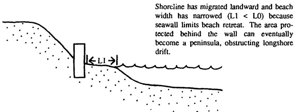
Figure 21. Long term effects of a seawall on a retreating shoreline
