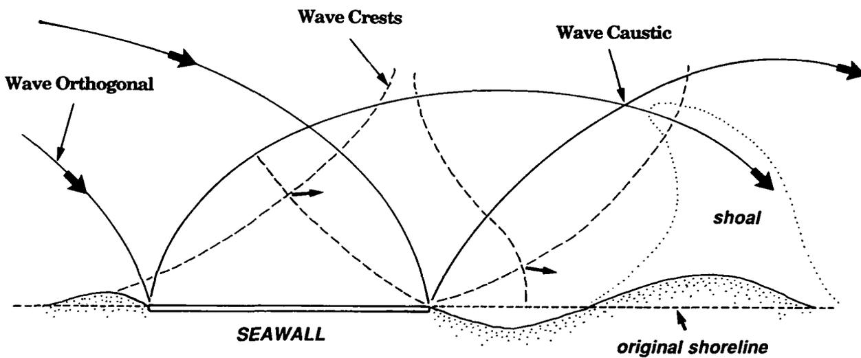
Figure 18. Short-crested wave system generated by obliquely reflected waves summing with incident waves. Areas of scour are produced in the vicinity of the wall and deposition occurs further downcoast. (From Silvester 1977)
