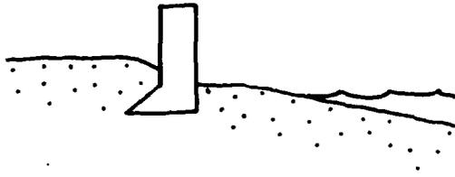
Seawall is placed well seaward on beach profile; a narrow summer berm exists. The beach in front of the wall is very sensitive to changes in sediment supply or sea level.
