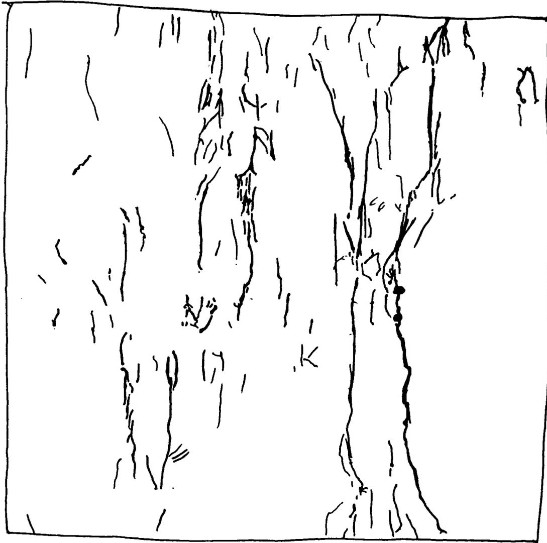
Figure 17b. Trace of dominant microcracks shown on the photomicrograph in Figure 17a.
