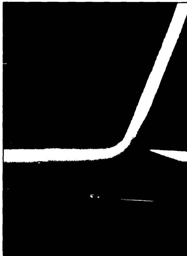
Figure 2. Scanning electron microscope picture of the top of such a wall, showing the extremely smooth and straight faces produced by the anisotropic etching.
