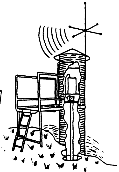
Remote Site Stream Gauge
