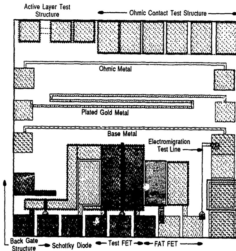
Figure 2. Test Element Group Used for Metallization Evaluation
