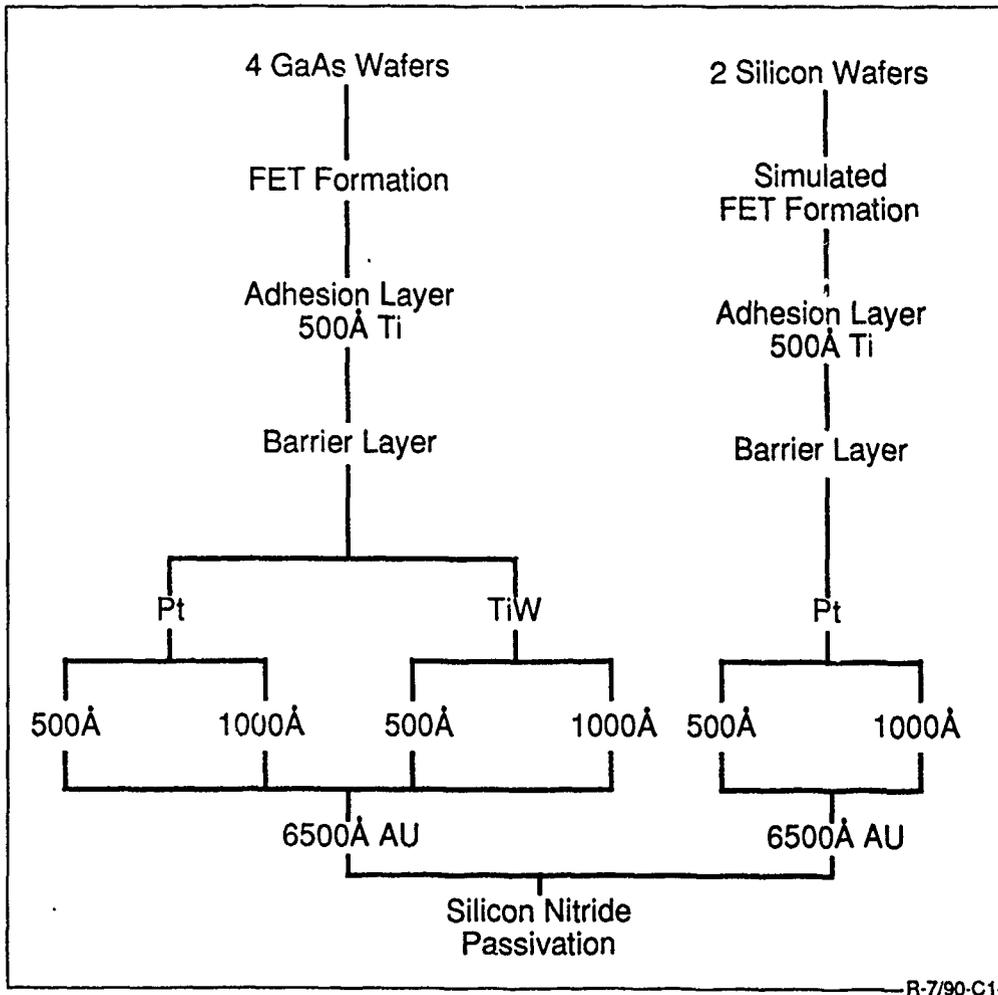
Figure 4. Wafer Process Flow With Barrier Metal Variations
