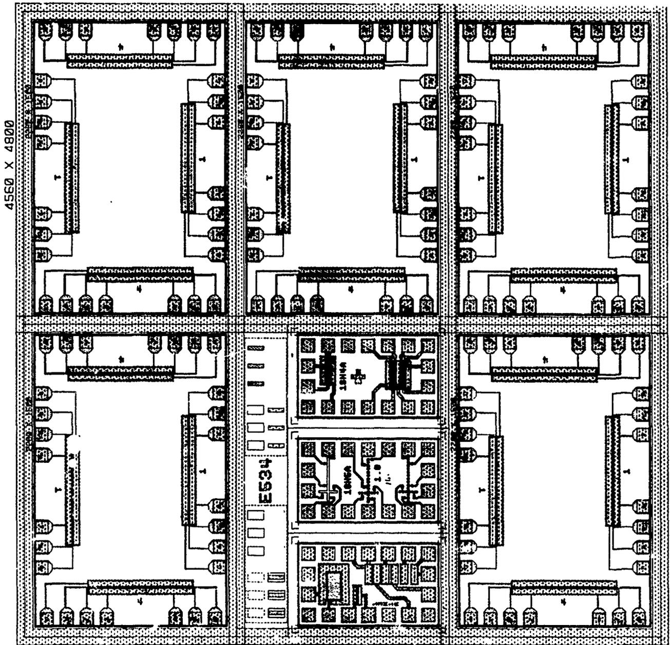
Figure 3. CALMA Plot of Electromigration Test Circuit Cluster
