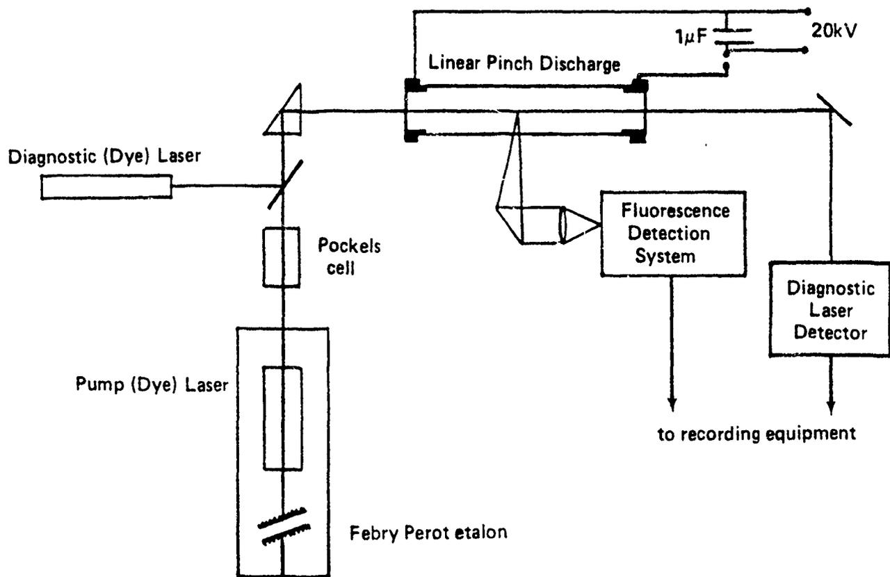
Figure C.1: Setup for LIF Experiment by Burgess *et al.*, (1980)
