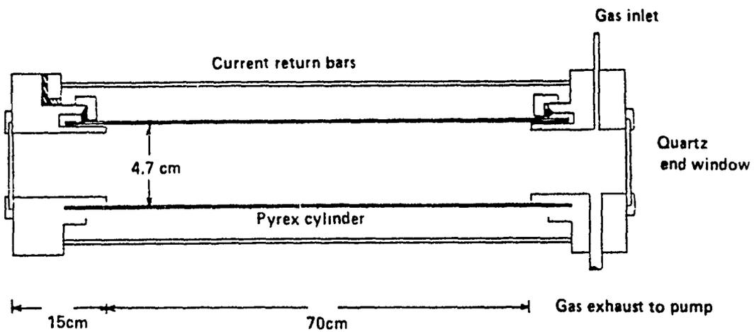
Figure D.2: Z-Pinch Plasma Vessel
