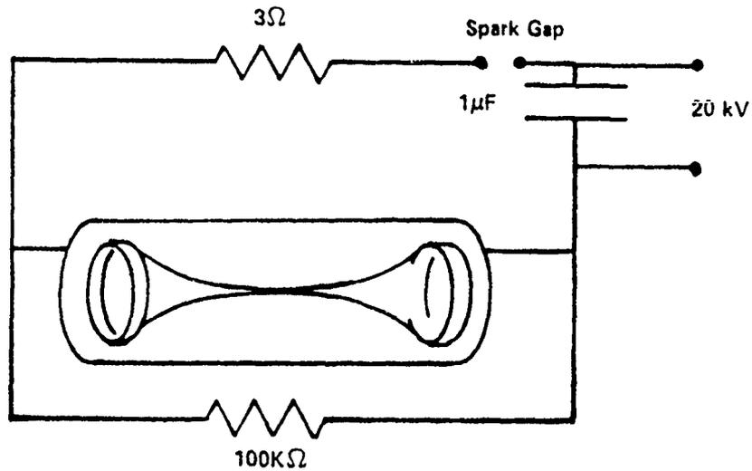
Figure D.1: Electrical Circuit for Z-Pinch
