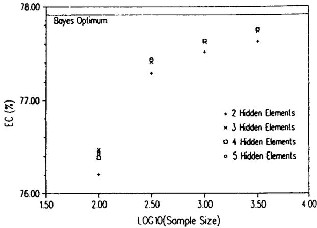
Fig. 2a. Mean values of the expected rate of correct classification plotted against training set size, for networks trained on the Gaussian classification problem.
