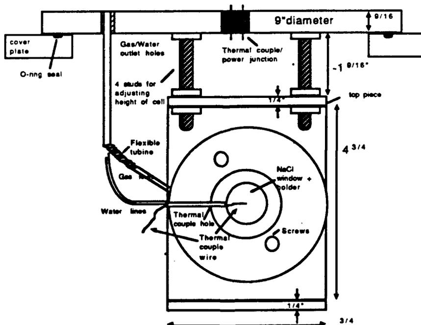
Figure 2-8: PORTABLE GAS HANDLING SYSTEM FOR PYRIDINE INFRARED SPECTROSCOPY STUDIES<sup>88</sup>
