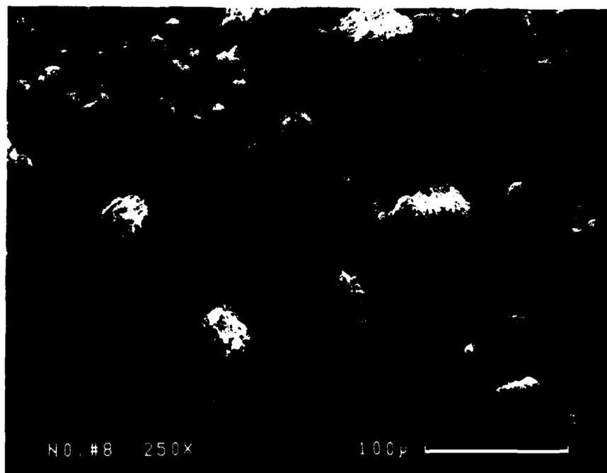
**Figure 3-9: SEM MICROGRAPH OF HEAT TREATED A-Nb<sub>2</sub>O<sub>5</sub> (800,2)**
