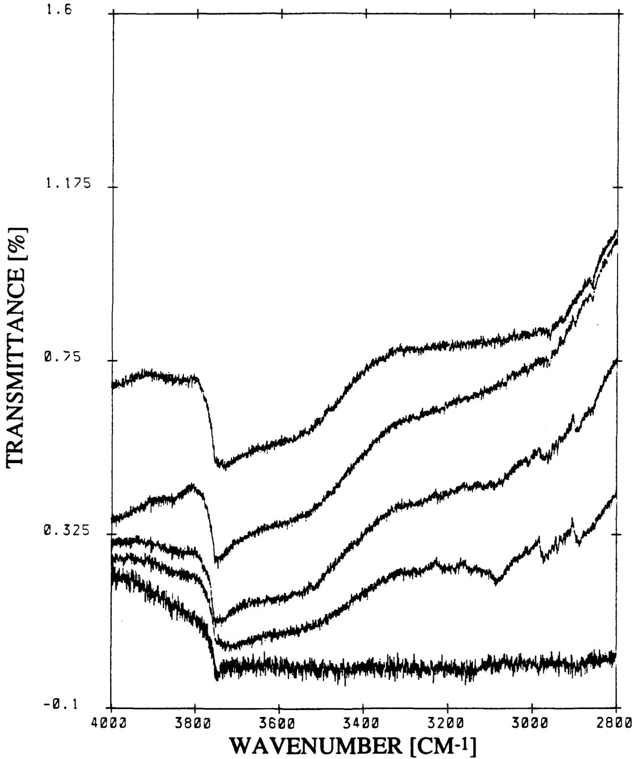
**Figure C-15:** HYDROXYL RANGE FTIR SPECTRA OF PYRIDINE ADSORBED ON A-NA25w: BLANK AND AFTER HEAT TREATMENTS AT 300, 200, AND 100 °C (TOP TO BOTTOM)
