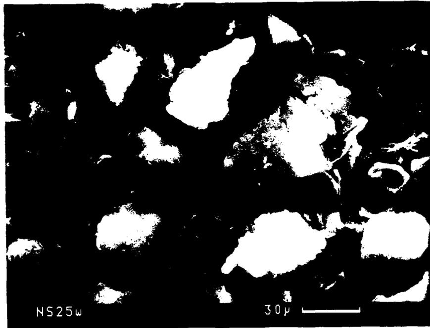
**Figure 4-11: NIOBIUM DOT MAP FOR A-NS25w (500,2)**
