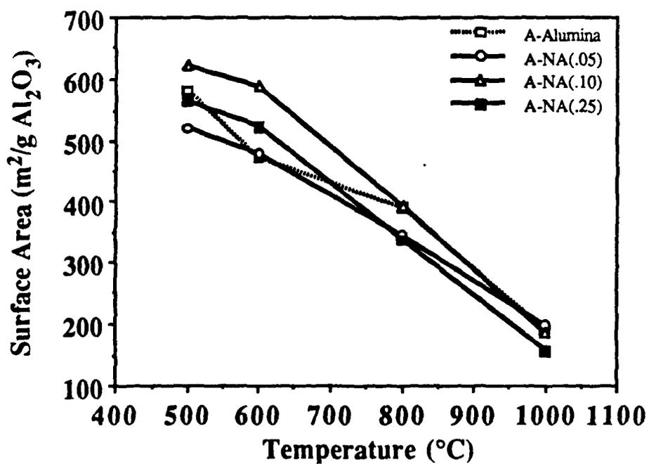
Figure 5-4: ALUMINA AEROGEL SUPPORTED NIOBIA NORMALIZED SURFACE AREA VS. TEMPERATURE
