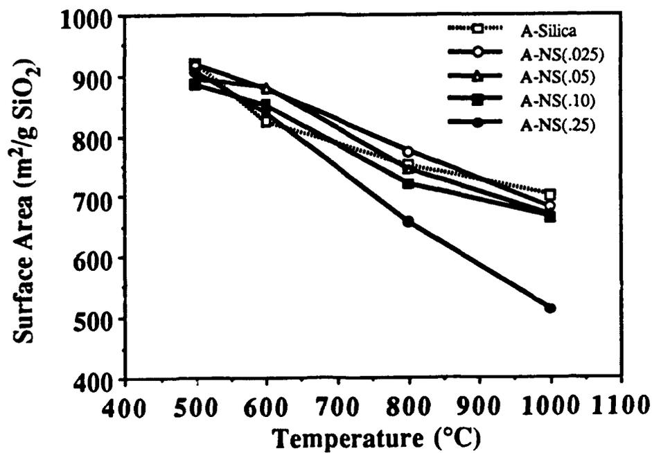
Figure 5-2: SILICA AEROGEL SUPPORTED NIOBIA NORMALIZED SURFACE AREA VS. TEMPERATURE
