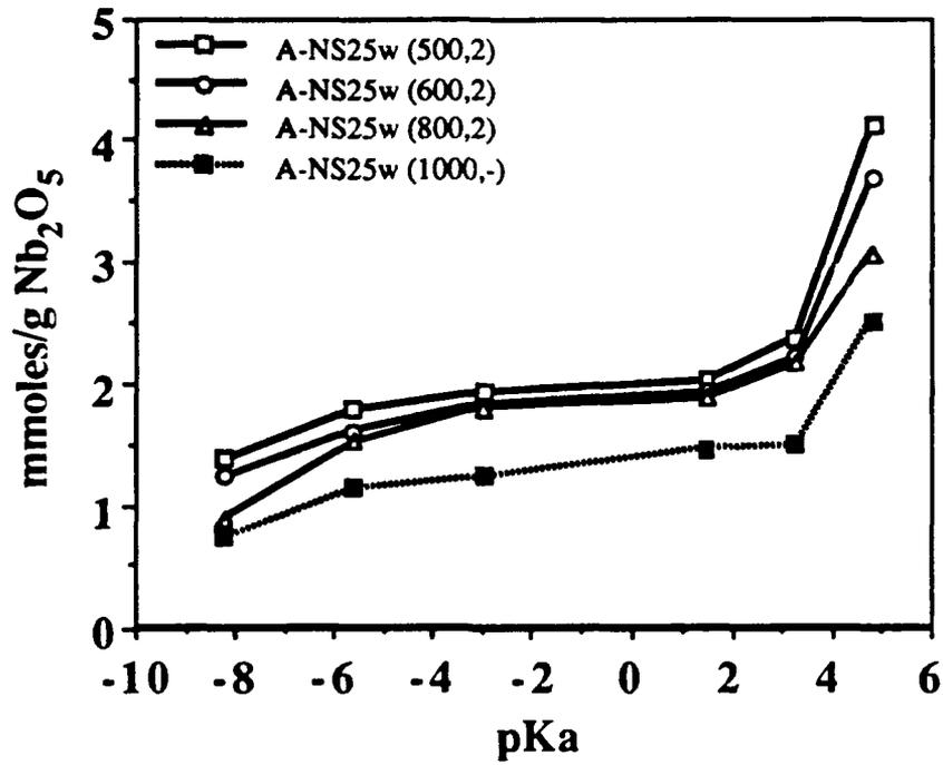
Figure 4-24: A-NS25W HEAT TREATED ACIDITY (MMOLES/M<sup>2</sup>) VS. pKa
