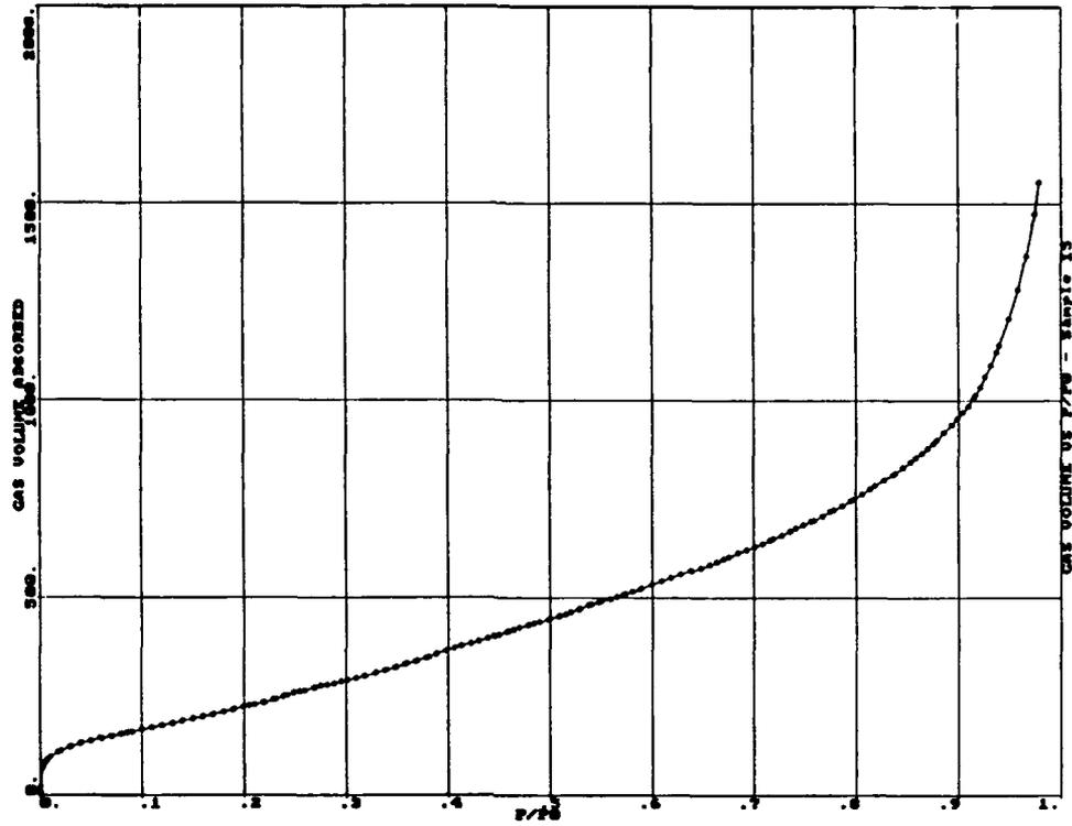
Figure B-12: PORE SIZE DISTRIBUTION FOR A-SiO<sub>2</sub> AS DETERMINED BY NITROGEN ADSORPTION
