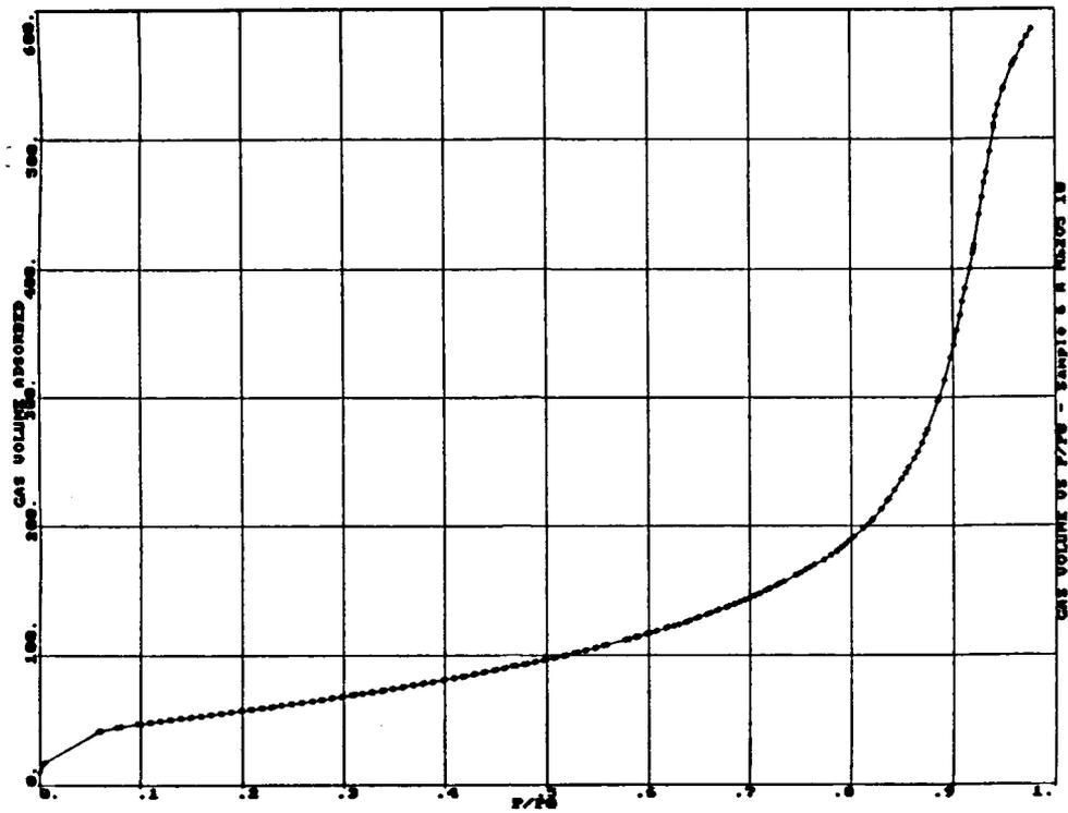
Figure B-44: PORE SIZE DISTRIBUTION FOR A-Nb<sub>2</sub>O<sub>5</sub> (0.31,10.,0.25) WITH MEOH AS DETERMINED BY NITROGEN ADSORPTION
