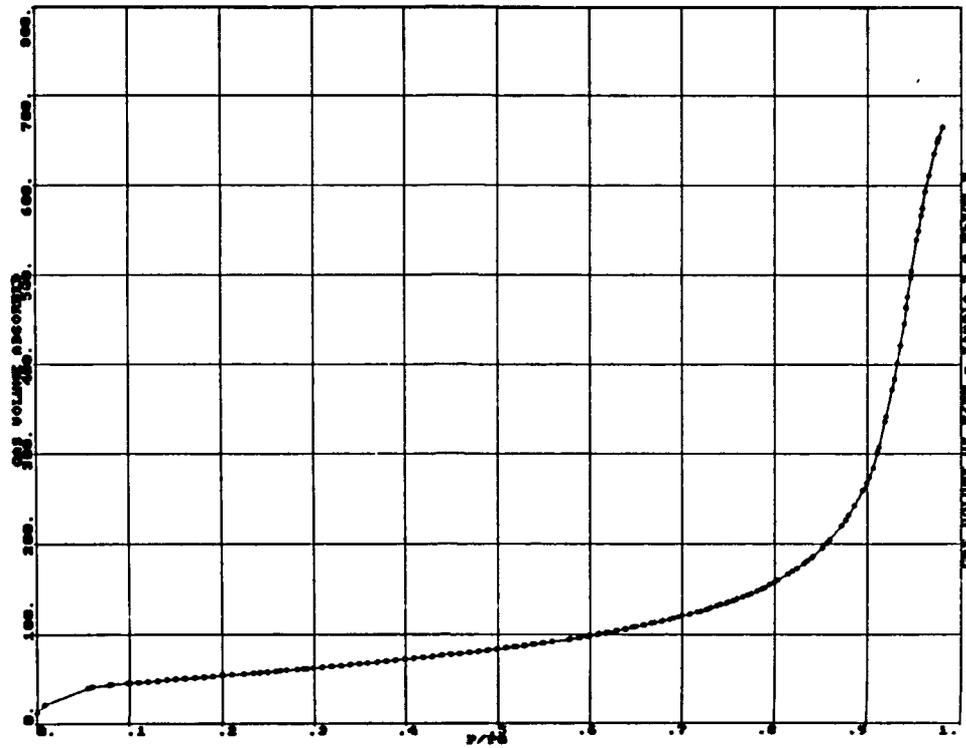
Figure B-42: PORE SIZE DISTRIBUTION FOR A-Nb<sub>2</sub>O<sub>5</sub> (0.50,10.,0.25) WITH MEOH AS DETERMINED BY NITROGEN ADSORPTION
