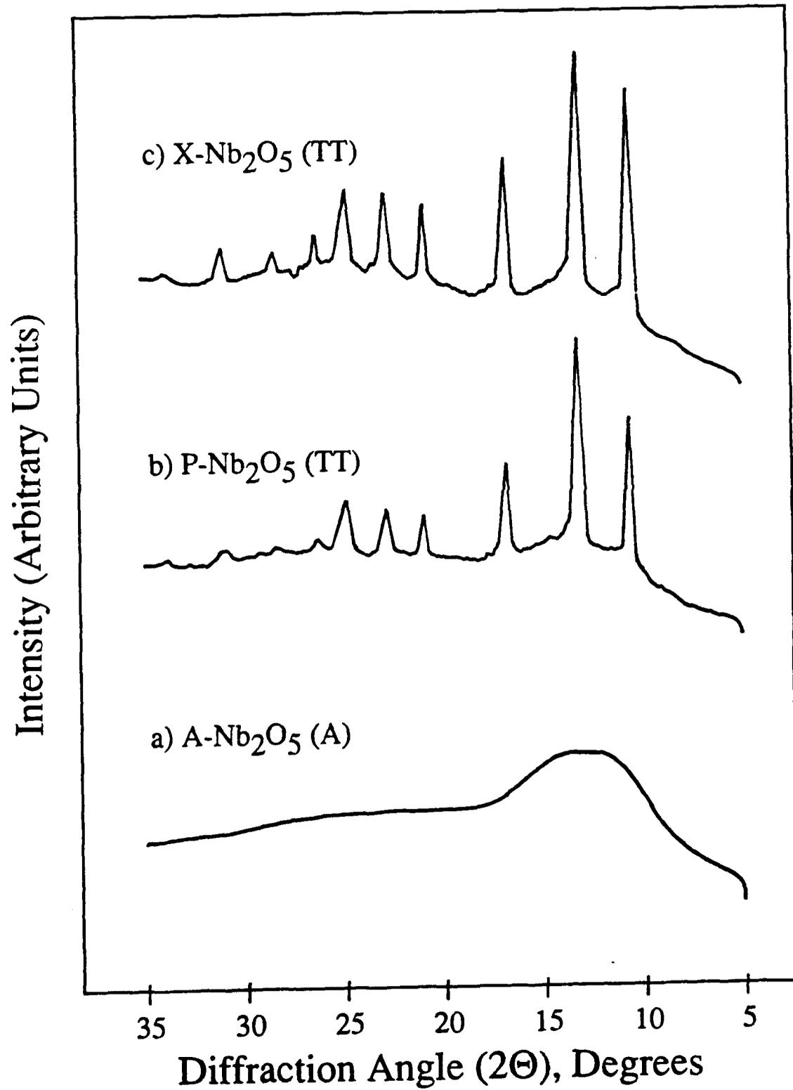
Figure 3-3: AMORPHOUS TO TT-Nb<sub>2</sub>O<sub>5</sub> TRANSITION OF CALCINED A-Nb<sub>2</sub>O<sub>5</sub> USING PLATINUM HOTSTAGE
