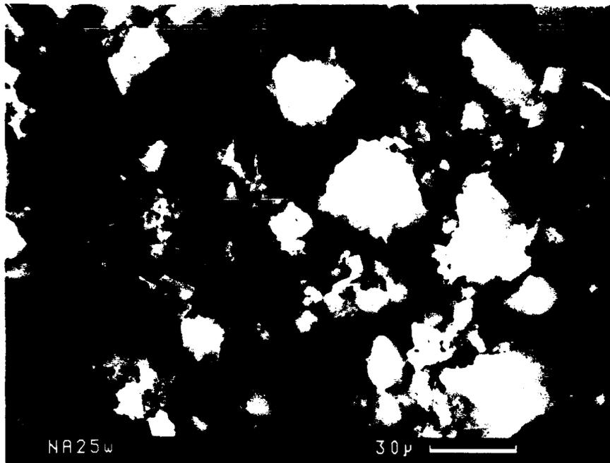
**Figure 4-14: NIOBIUM DOT MAP FOR A-NA25w (500,2)**
