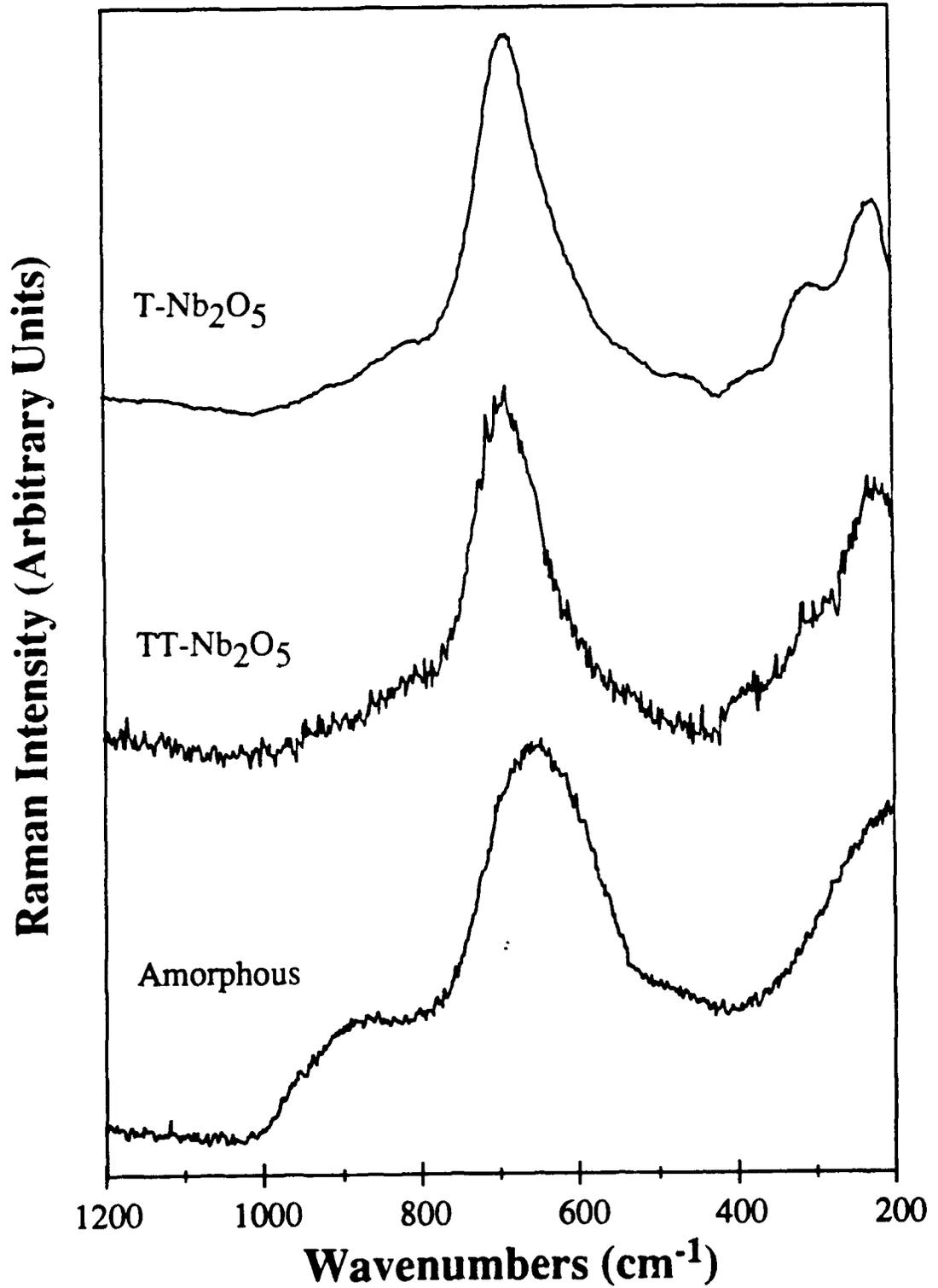
Figure 3-14: LRS SPECTRA OF A-Nb<sub>2</sub>O<sub>5</sub> AFTER HEAT TREATMENT: (800,2) [T], (1000,-) [M], AND (1000,8) [H] (FROM BOTTOM TO TOP)
