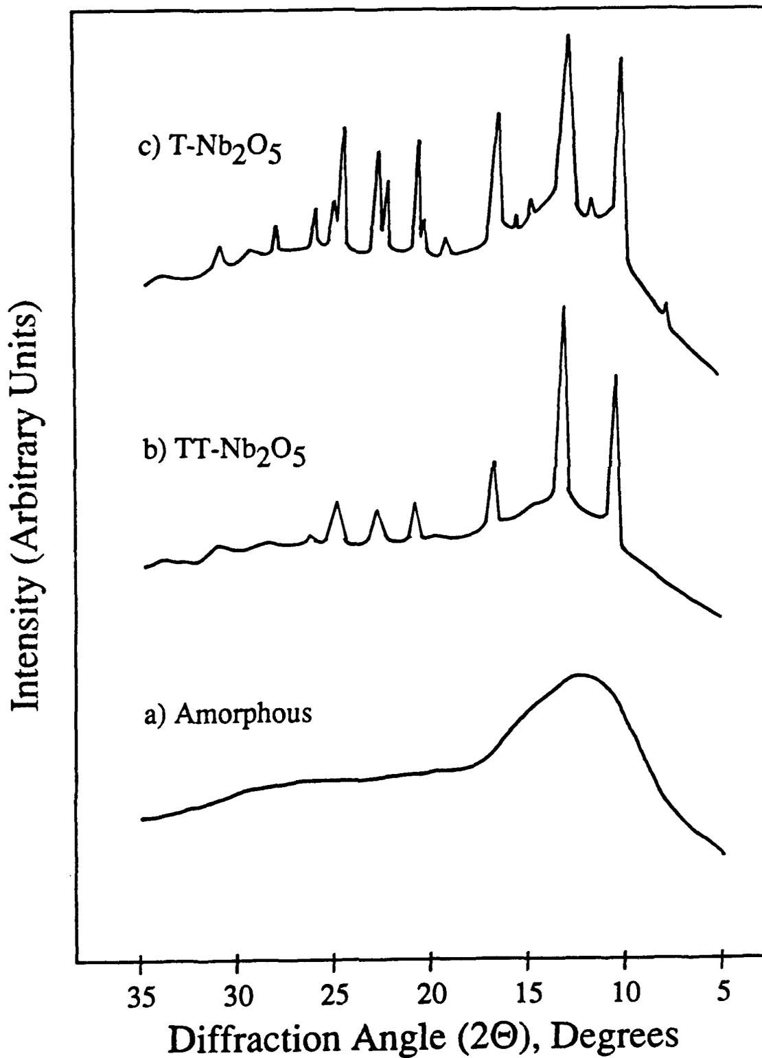
Figure 3-5: XRD OF A-Nb<sub>2</sub>O<sub>5</sub> AFTER HEAT TREATMENT: A) (800,2) [T], B) (1000,-) [M], AND C) (1000,8) [H] (NIOBIA PHASE IN BRACKETS)
