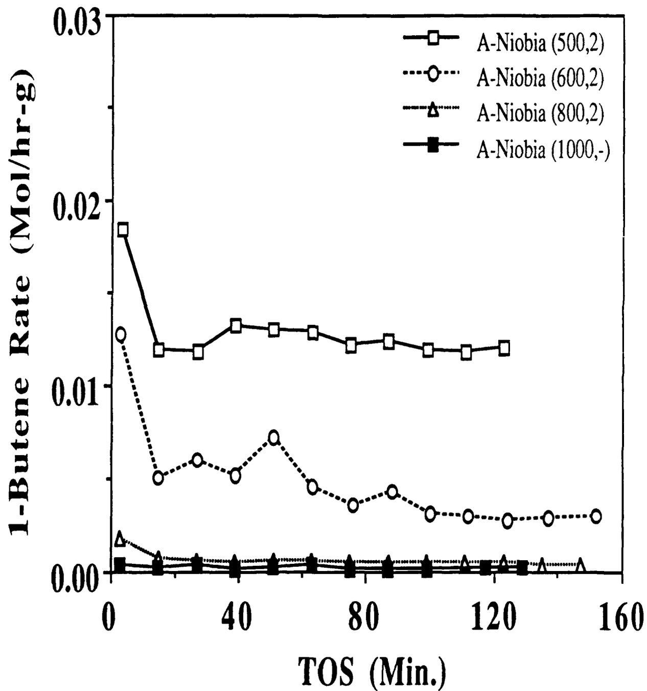
Figure 3-28: 1-BUTENE ISOMERIZATION ACTIVITY OVER HEAT TREATED A-Nb<sub>2</sub>O<sub>5</sub> (M<sup>2</sup>)
