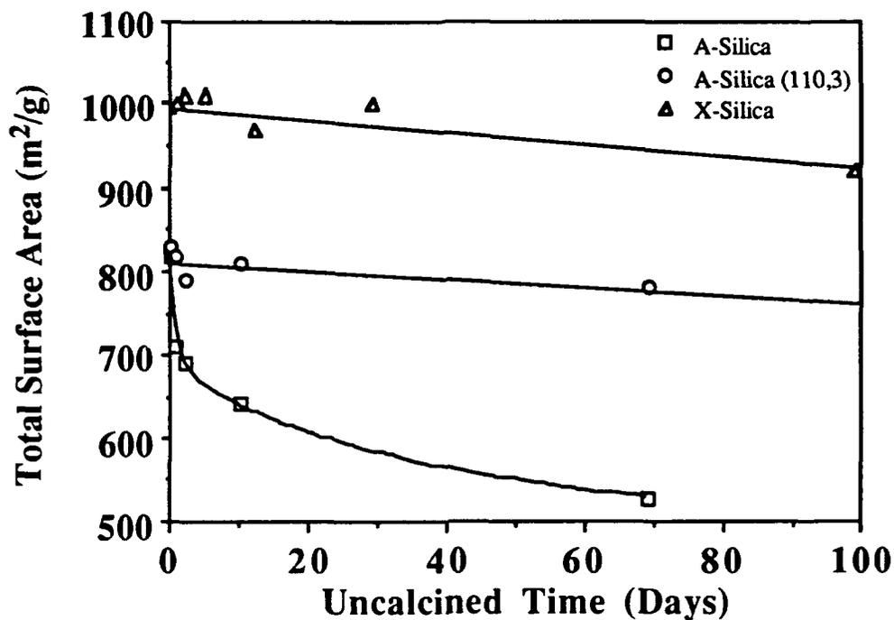
Figure D-2: A-SiO<sub>2</sub> AND X-SiO<sub>2</sub> NORMALIZED SURFACE AREA STABILITY VERSUS UNCALCINED TIME
