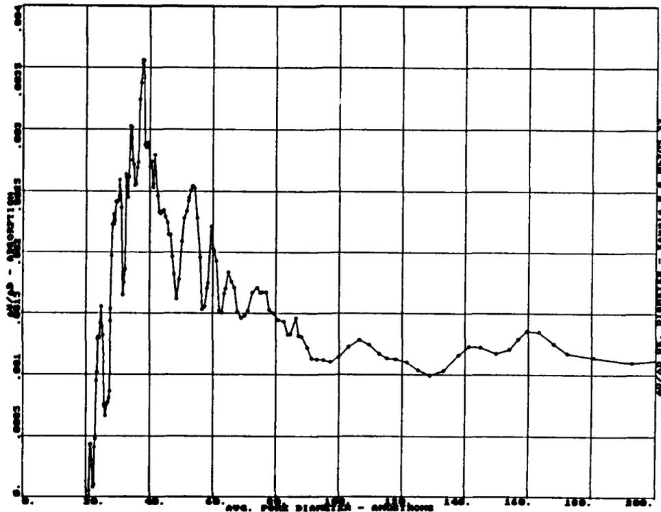
Figure B-49: NITROGEN DESORPTION ISOTHERM OF A-Nb<sub>2</sub>O<sub>5</sub> (0.31,5.,0.80) WITH S-BUOH
