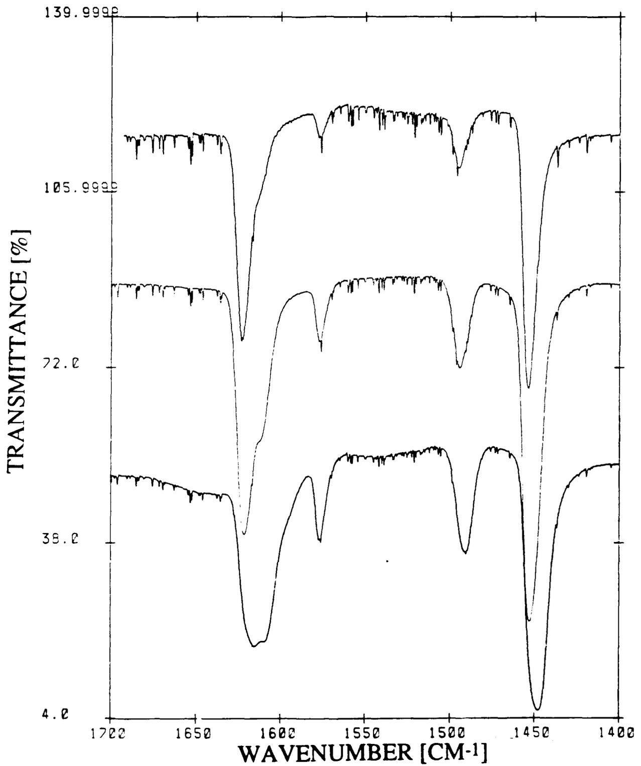
Figure 4-31: FTIR SPECTRA OF PYRIDINE ADSORBED ON NA25w AFTER HEAT TREATMENTS AT 300, 200, AND 100 °C (TOP TO BOTTOM)
