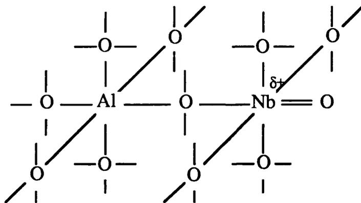
**Figure 6-9:** PROPOSED MOLECULAR STRUCTURE FOR A-NA25w AFTER A (500,2) CALCINATION
