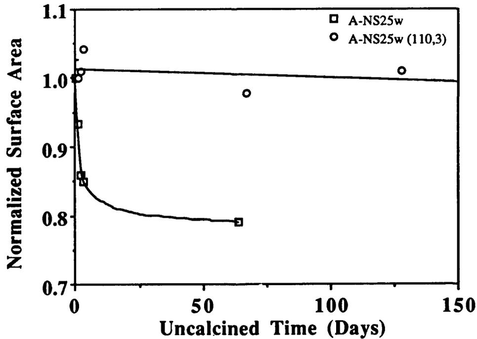
Figure D-5: A-NS25w TOTAL SURFACE AREA STABILITY VERSUS UNCALCINED TIME
