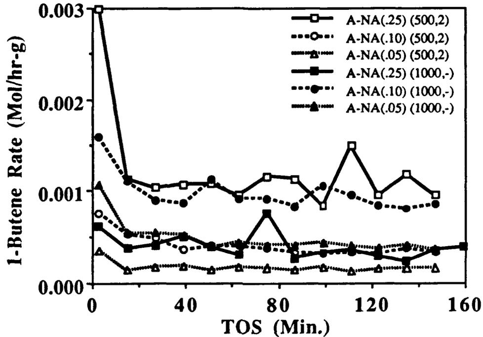
Figure 5-42: 1-BUTENE ISOMERIZATION ACTIVITY (/G Nb<sub>2</sub>O<sub>5</sub>) OVER HEAT TREATED ALUMINA AEROGEL SUPPORTED NIOBIA
