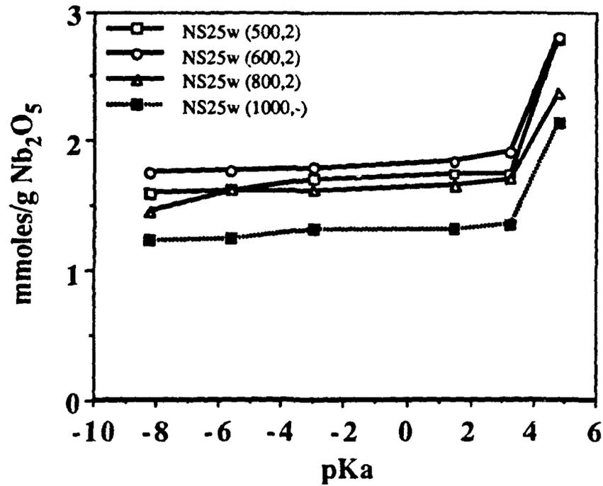
Figure 4-26: NS25W HEAT TREATED ACIDITY (MMOLES/M<sup>2</sup>) VS. pKa
