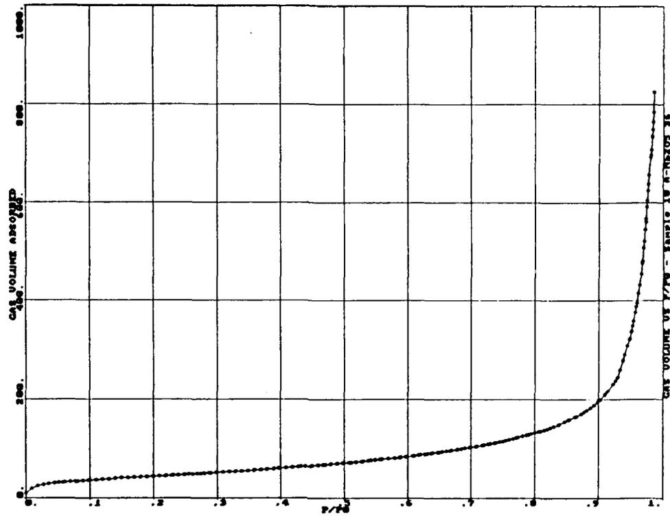
Figure B-52: PORE SIZE DISTRIBUTION FOR A-Nb<sub>2</sub>O<sub>5</sub> (0.625,10.,0.80) WITH S-BUOH AS DETERMINED BY NITROGEN ADSORPTION
