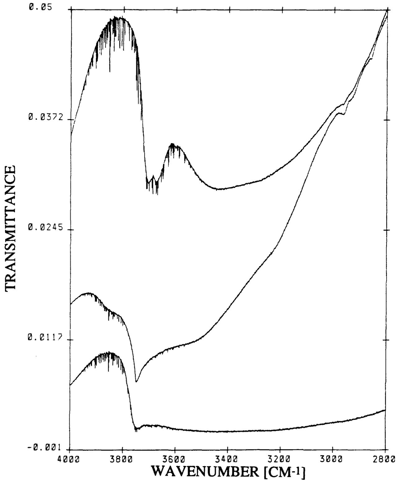
Figure C-22: DRIFT HYDROXYL RANGE SPECTRA FOR CALCINED (500,2): A-Nb<sub>2</sub>O<sub>5</sub>, A-NS25w, AND A-SiO<sub>2</sub> (TOP TO BOTTOM)
