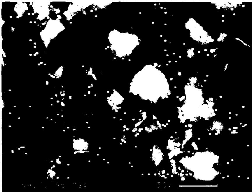
**Figure 4-15: ALUMINUM DOT MAP FOR A-NA25w (500,2)**
