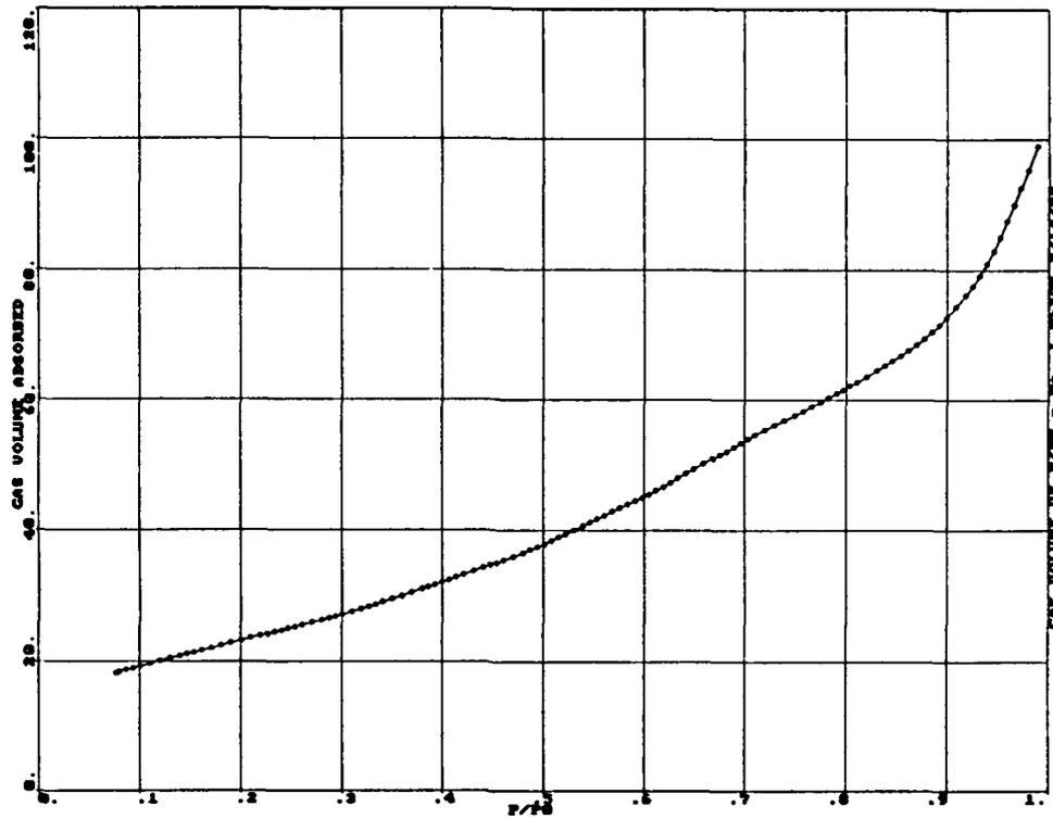
Figure B-4: PORE SIZE DISTRIBUTION FOR P-Nb<sub>2</sub>O<sub>5</sub> AS DETERMINED BY NITROGEN ADSORPTION
