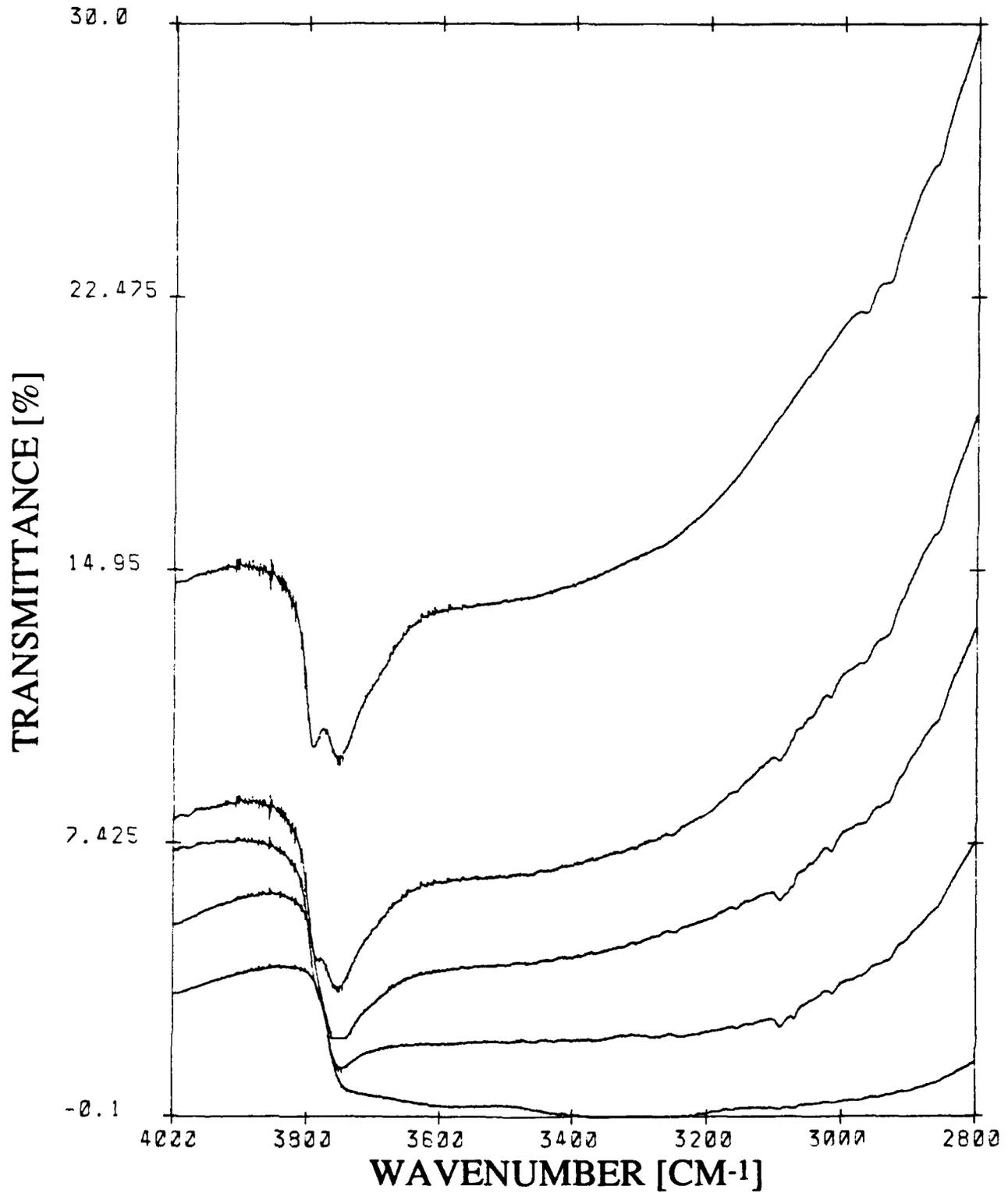
**Figure C-19:** HYDROXYL RANGE FTIR SPECTRA OF PYRIDINE ADSORBED ON A-NA(.25): BLANK AND AFTER HEAT TREATMENTS AT 300, 200, 100, AND 25 °C (TOP TO BOTTOM)
