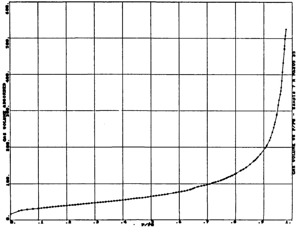
Figure B-46: PORE SIZE DISTRIBUTION FOR A-Nb<sub>2</sub>O<sub>5</sub> (0.625,5.,0.80) WITH S-BUOH AS DETERMINED BY NITROGEN ADSORPTION
