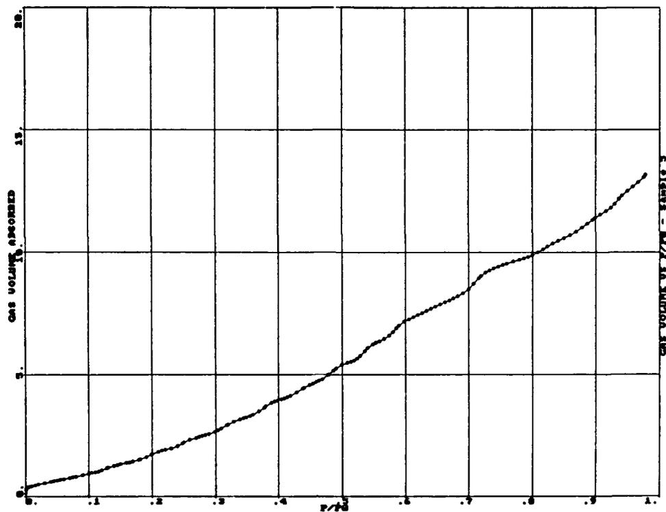
Figure B-30: PORE SIZE DISTRIBUTION FOR P-Nb<sub>2</sub>O<sub>5</sub> (1000,-) AS DETERMINED BY NITROGEN ADSORPTION
