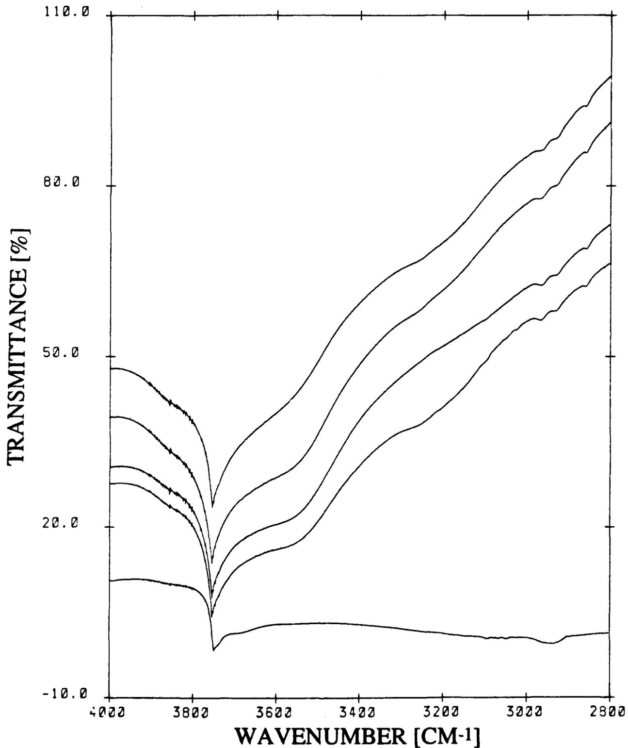
**Figure C-13: HYDROXYL RANGE FTIR SPECTRA OF PYRIDINE ADSORBED ON  $\alpha$ - $\text{Al}_2\text{O}_3$ : BLANK AND AFTER HEAT TREATMENTS AT 300, 200, 100, AND 25 °C (TOP TO BOTTOM)**
