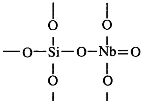
**Figure 6-5:** PROPOSED MOLECULAR STRUCTURE FOR A-NS25w AFTER A (500,2) CALCINATION
