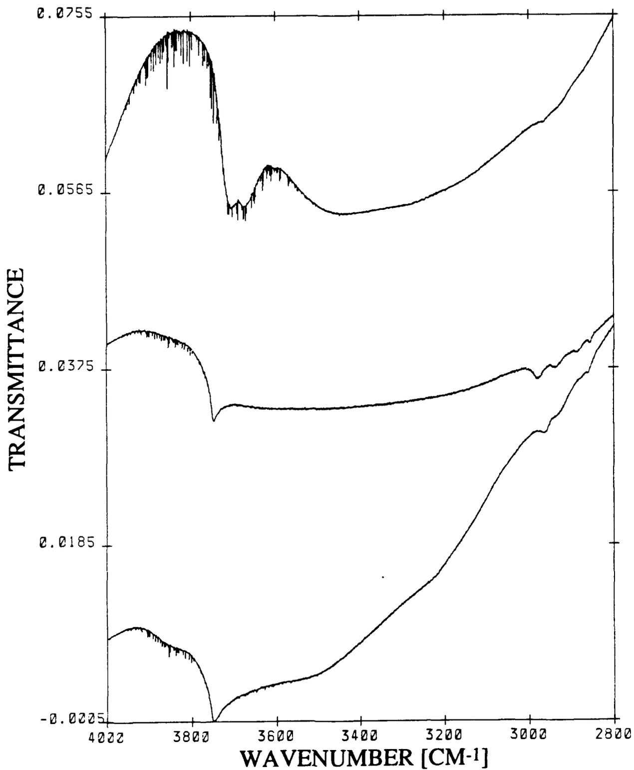
water as shown by the strong absorption throughout the range 3700 to 3000  $\text{cm}^{-1}$ . The hydroxyl region shows a single peak at 3749  $\text{cm}^{-1}$  which is probably attributed to the large amount of silica found in this oxide, and the second hydroxyl peak observed in the FTIR of this oxide is probably obscured by the strong absorption of chemisorbed water. This is similar to the effect that pyridine was found to have on this mixed oxide.
