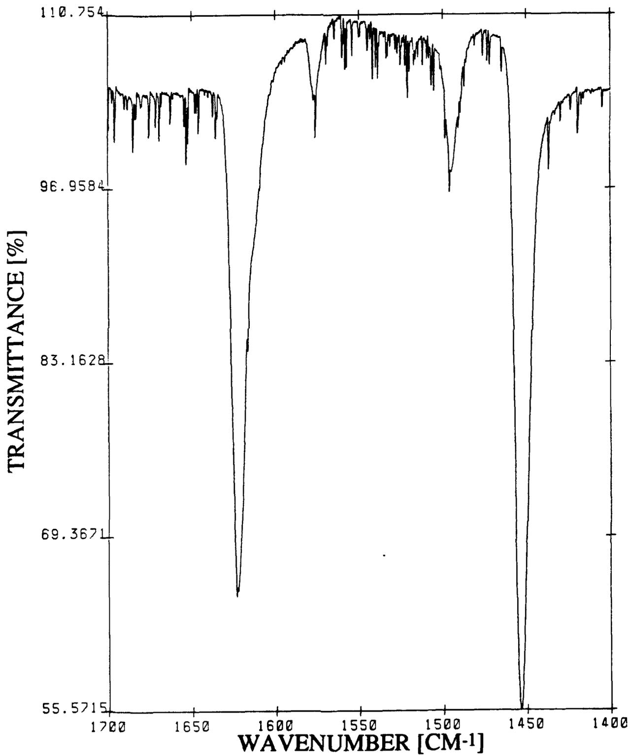
Figure C-6: FTIR SPECTRUM OF PYRIDINE ADSORBED ON NA25w AFTER HEAT TREATMENT AT 300 °C
