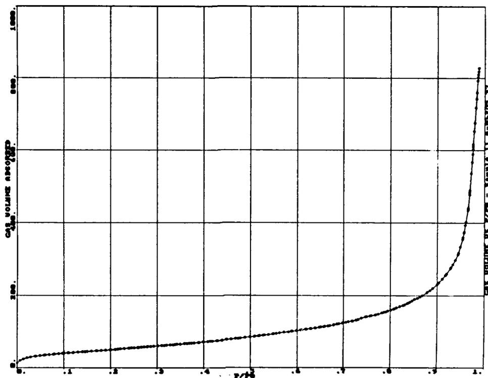
Figure B-54: PORE SIZE DISTRIBUTION FOR A-Nb<sub>2</sub>O<sub>5</sub> (0.50,10.,0.80) WITH S-BUOH AS DETERMINED BY NITROGEN ADSORPTION
