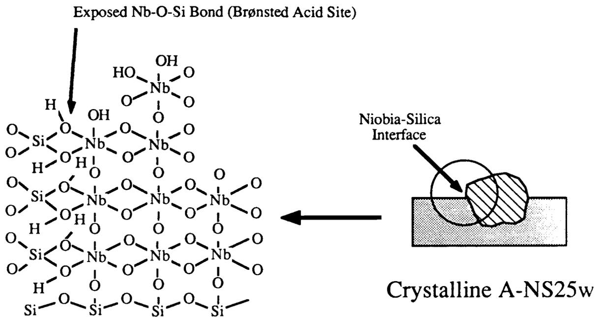
**Figure 6-13: PROPOSED MOLECULAR STRUCTURE FOR OCTAHEDRAL NIOBIA-RIGID SILICA INTERFACE IN A-NS(.25)**
