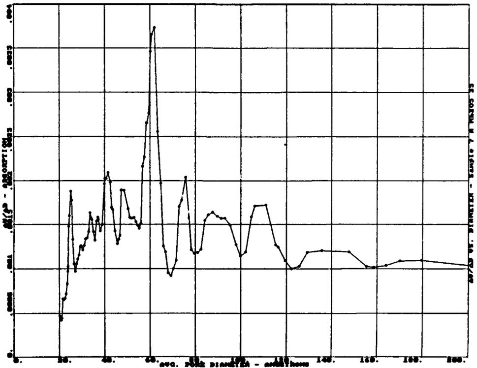
Figure B-47: NITROGEN DESORPTION ISOTHERM OF A-Nb<sub>2</sub>O<sub>5</sub> (0.50,5.,0.80) WITH S-BUOH
