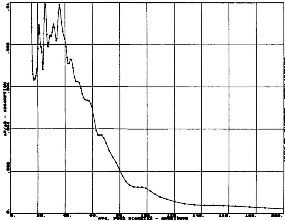
Figure B-21: NITROGEN DESORPTION ISOTHERM OF NA25w
