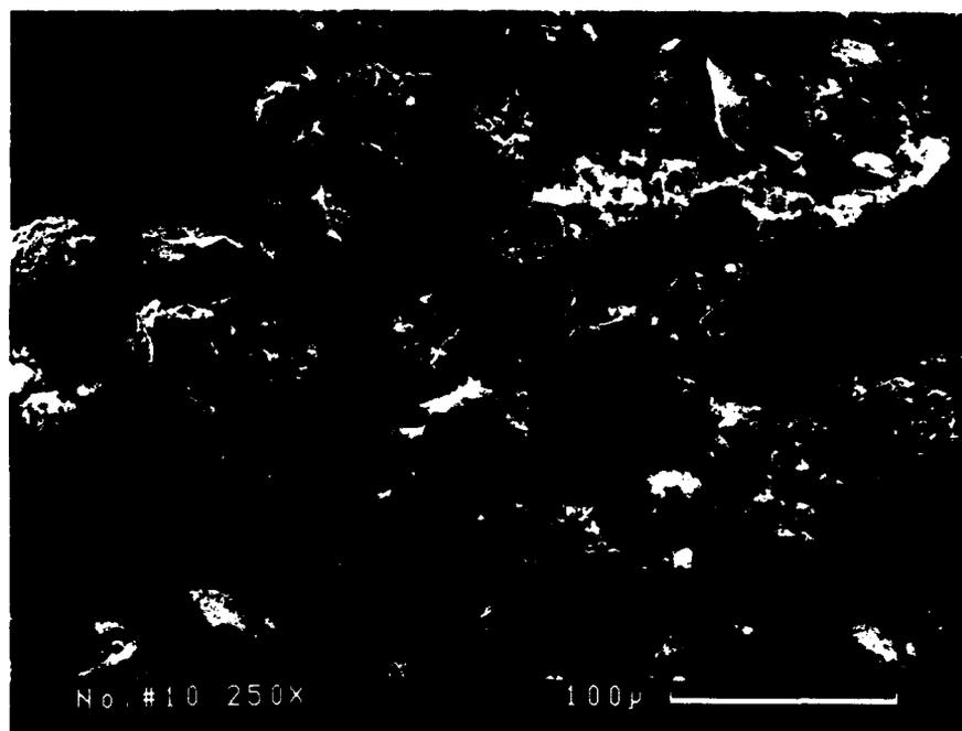
**Figure 3-11: SEM MICROGRAPH OF CALCINED X-Nb<sub>2</sub>O<sub>5</sub> (500,2)**
