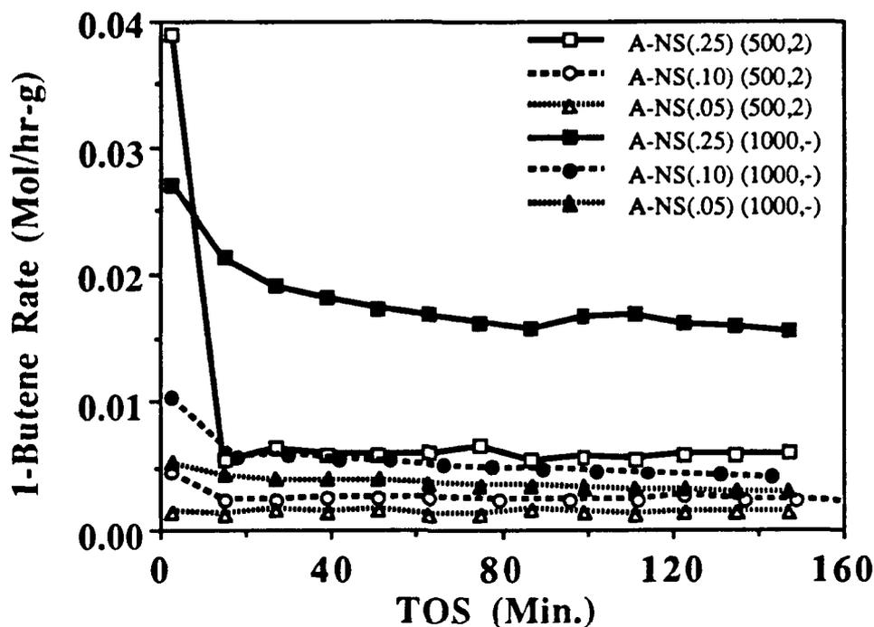
Figure 5-40: 1-BUTENE ISOMERIZATION ACTIVITY ( $\mu\text{G Nb}_2\text{O}_5$ ) OVER HEAT TREATED SILICA AEROGEL SUPPORTED NIOBIA
