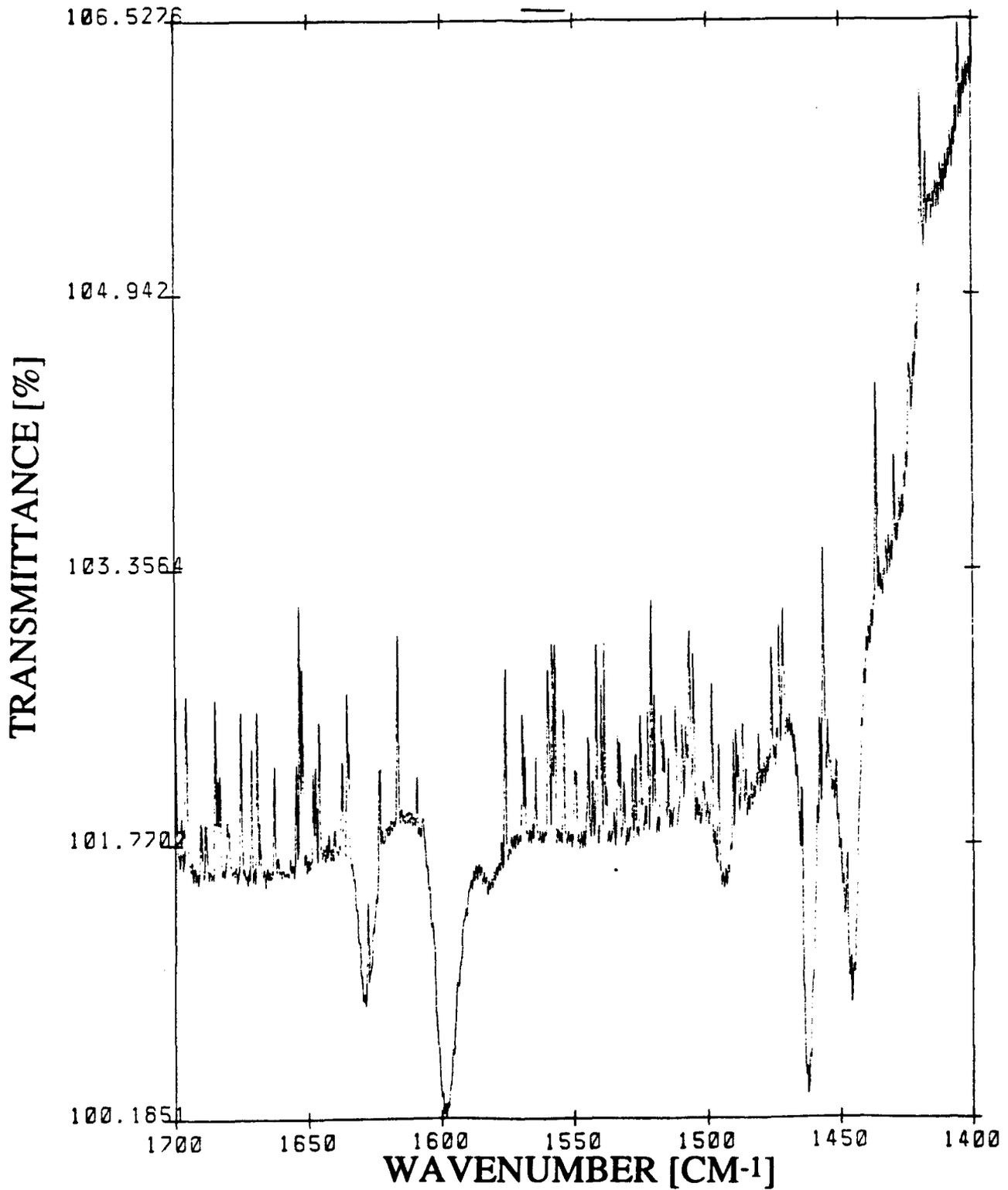
Figure C-3: FTIR SPECTRUM OF PYRIDINE ADSORBED ON  $\alpha$ - $\text{Al}_2\text{O}_3$  AFTER HEAT TREATMENT AT 300°C
