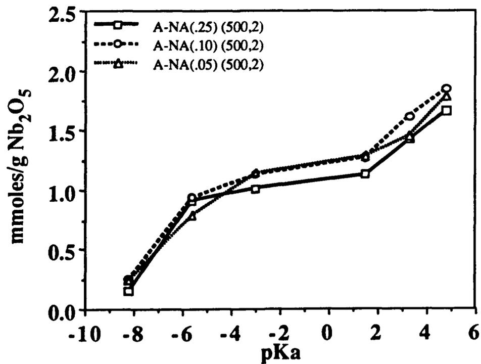
Figure 5-28: ALUMINA AEROGEL SUPPORTED NIOBIA ACIDITY (G Nb<sub>2</sub>O<sub>5</sub>)
