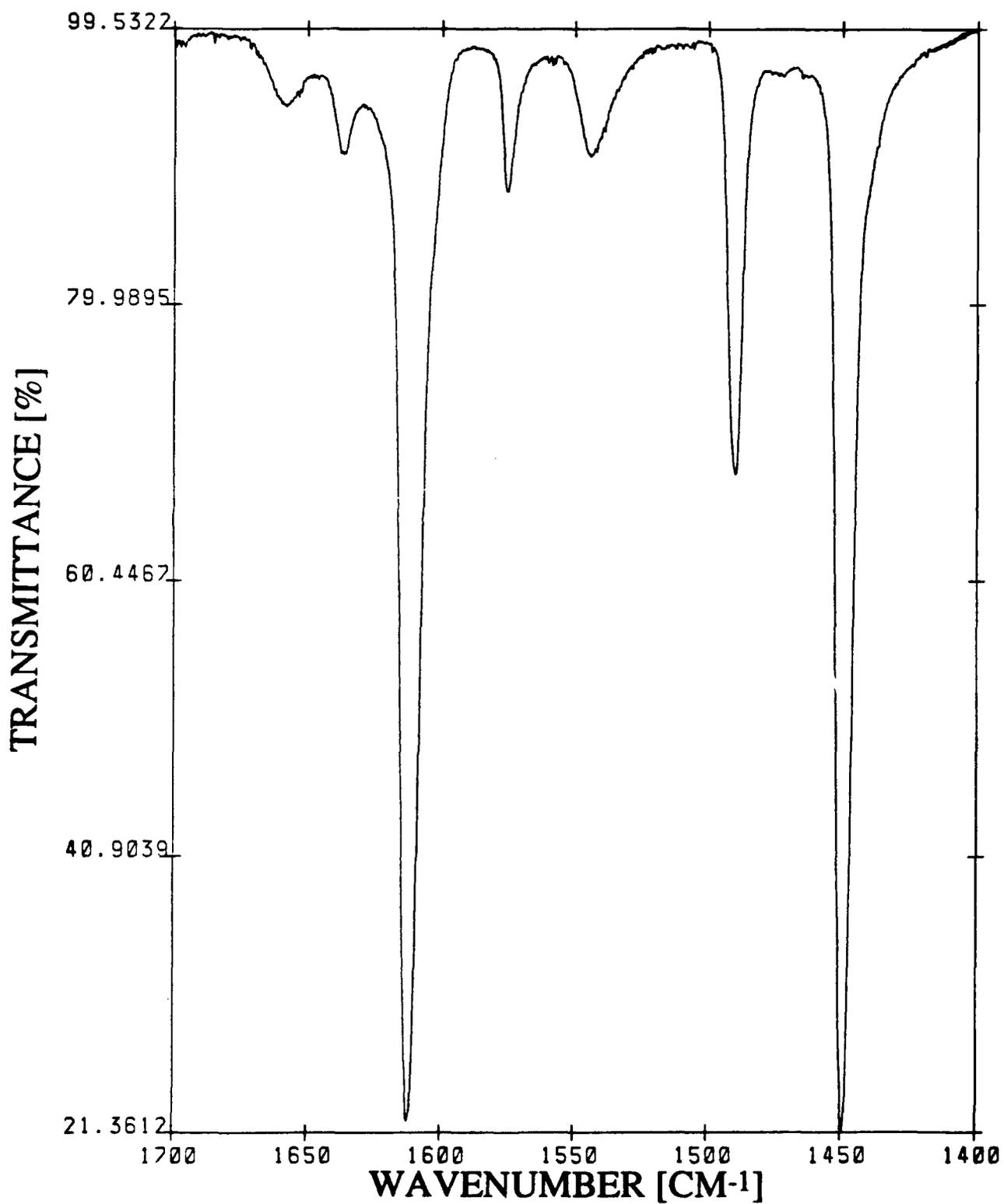
**Figure C-2: FTIR SPECTRUM OF PYRIDINE ADSORBED ON A-SiO<sub>2</sub> AFTER HEAT TREATMENT AT 300 °C**
