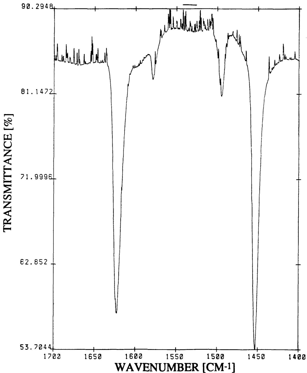
**Figure C-4: FTIR SPECTRUM OF PYRIDINE ADSORBED ON A-NS25w AFTER HEAT TREATMENT AT 300 °C**
