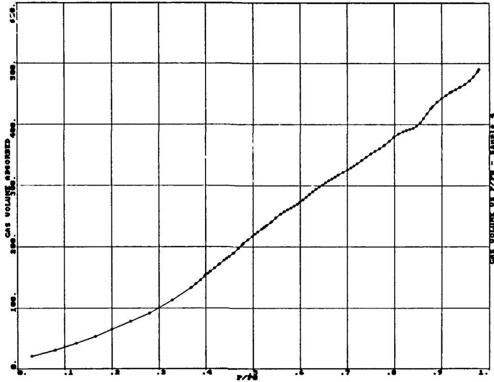
Figure B-28: PORE SIZE DISTRIBUTION FOR A-Nb<sub>2</sub>O<sub>5</sub> (1000,-) AS DETERMINED BY NITROGEN ADSORPTION
