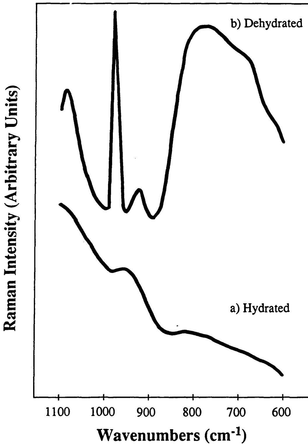
Figure 4-19: IN-SITU LRS SPECTRA OF A-NA25w (600,2): A) HYDRATED AND B) DEHYDRATED (450,30 min)
