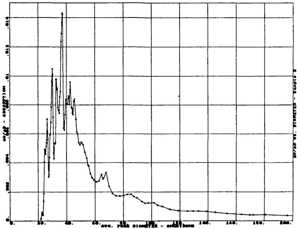
Figure B-25: NITROGEN DESORPTION ISOTHERM OF A-Nb<sub>2</sub>O<sub>5</sub> (800,2)
