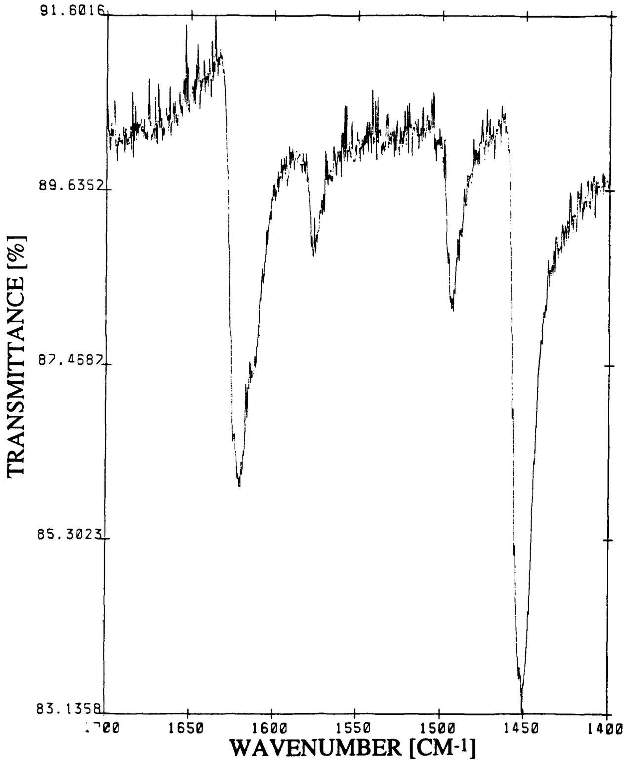
Figure C-7: FTIR SPECTRUM OF PYRIDINE ADSORBED ON A-NS(.05) AFTER HEAT TREATMENT AT 300 °C
