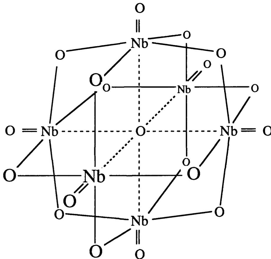
**Figure 6-3:** PROPOSED MOLECULAR STRUCTURE FOR CONVENTIONALLY PREPARED NIOBIA AFTER A (500,2) CALCINATION: BASIC BUILDING BLOCK IS A SLIGHTLY DISTORTED  $\text{NbO}_6$  OCTAHEDRON
