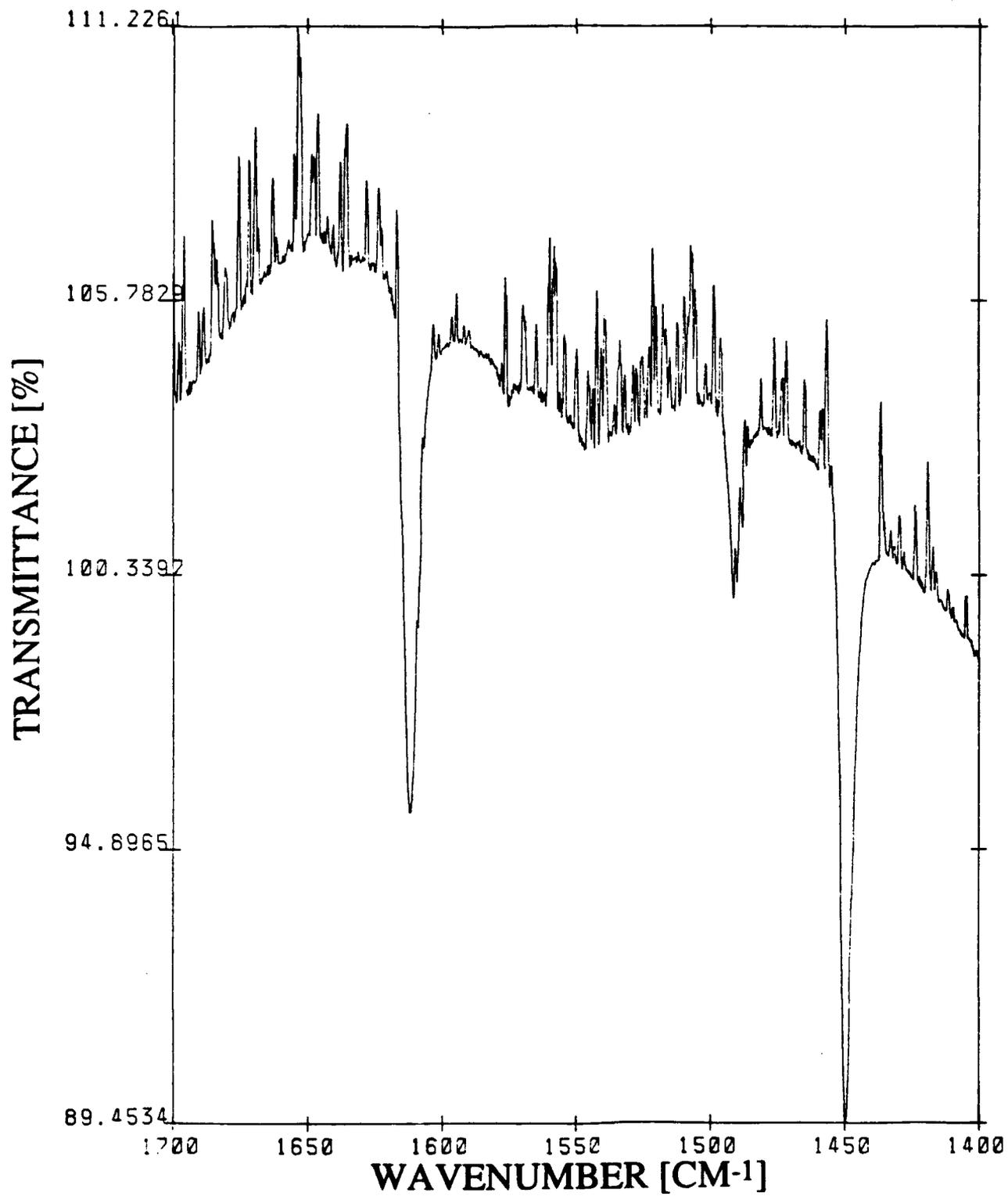
Figure C-8: FTIR SPECTRUM OF PYRIDINE ADSORBED ON A-NS(.25) AFTER HEAT TREATMENT AT 300 °C
