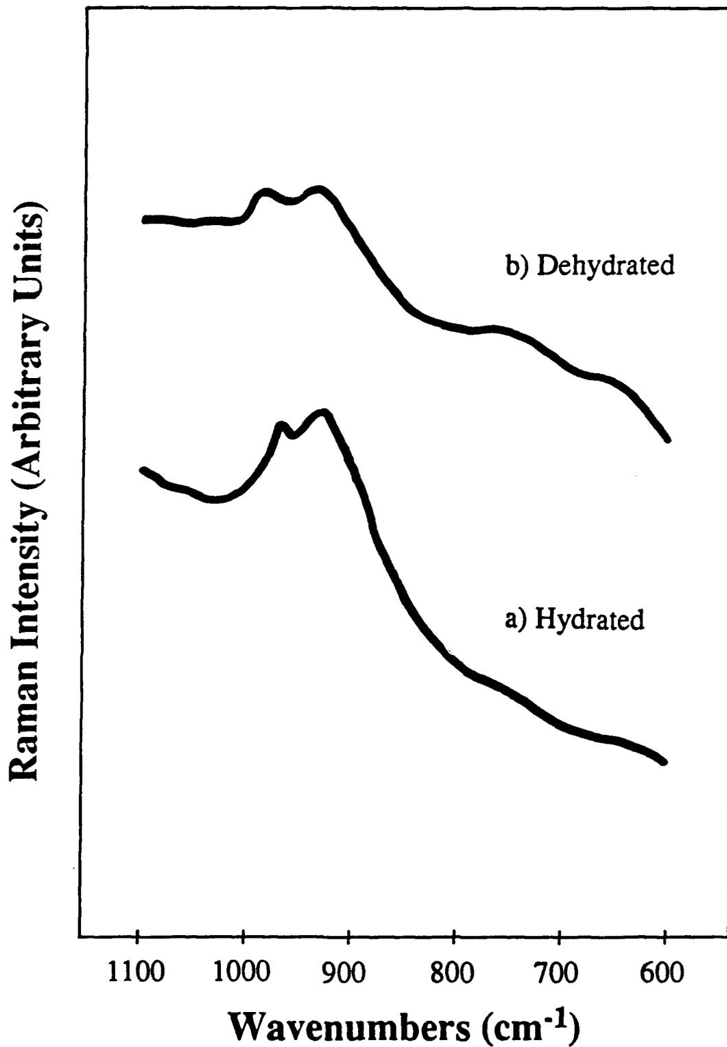
Figure 5-21: DRIFT SPECTRA OF A-NS(.25) AND A-SiO<sub>2</sub>
