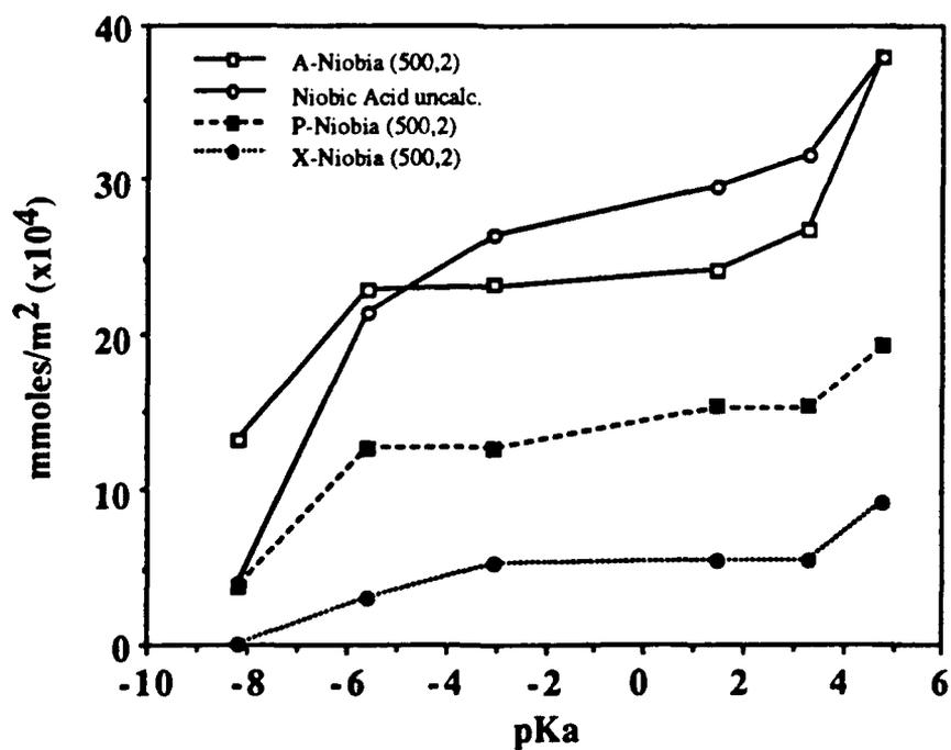
Figure 3-17: A) HEAT TREATED NIOBIA ACIDITY (MMOLES/G) AND B) HEAT TREATED NIOBIA ACIDITY (MMOLES/M<sup>2</sup>) VS. pKa
