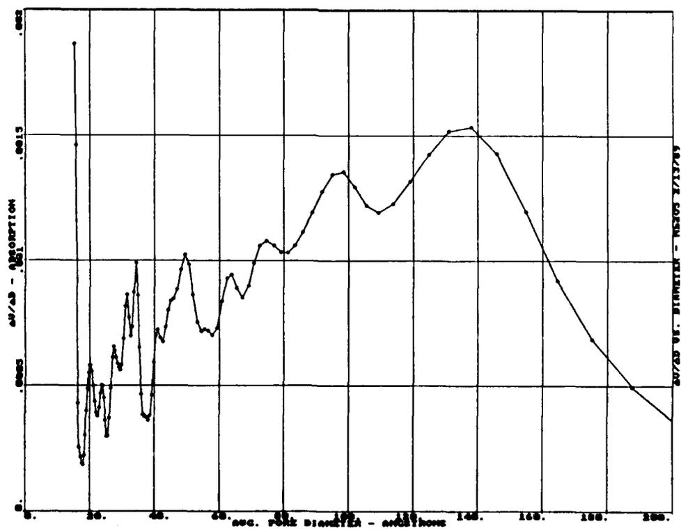
Figure B-7: NITROGEN DESORPTION ISOTHERM OF NIOBIC ACID
