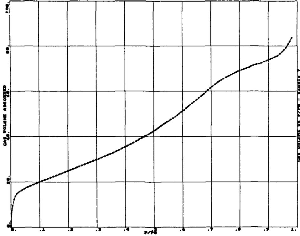
Figure B-8: PORE SIZE DISTRIBUTION FOR NIOBIC ACID AS DETERMINED BY NITROGEN ADSORPTION
