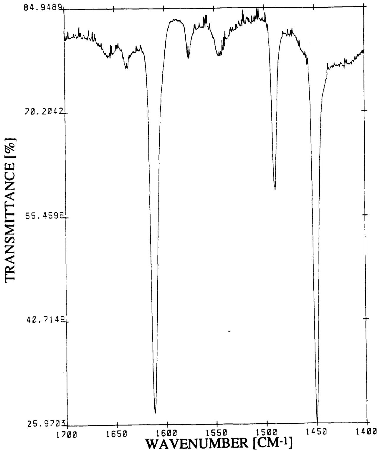
**Figure C-9:** FTIR SPECTRUM OF PYRIDINE ADSORBED ON A-NA(.05) AFTER HEAT TREATMENT AT 300 °C
