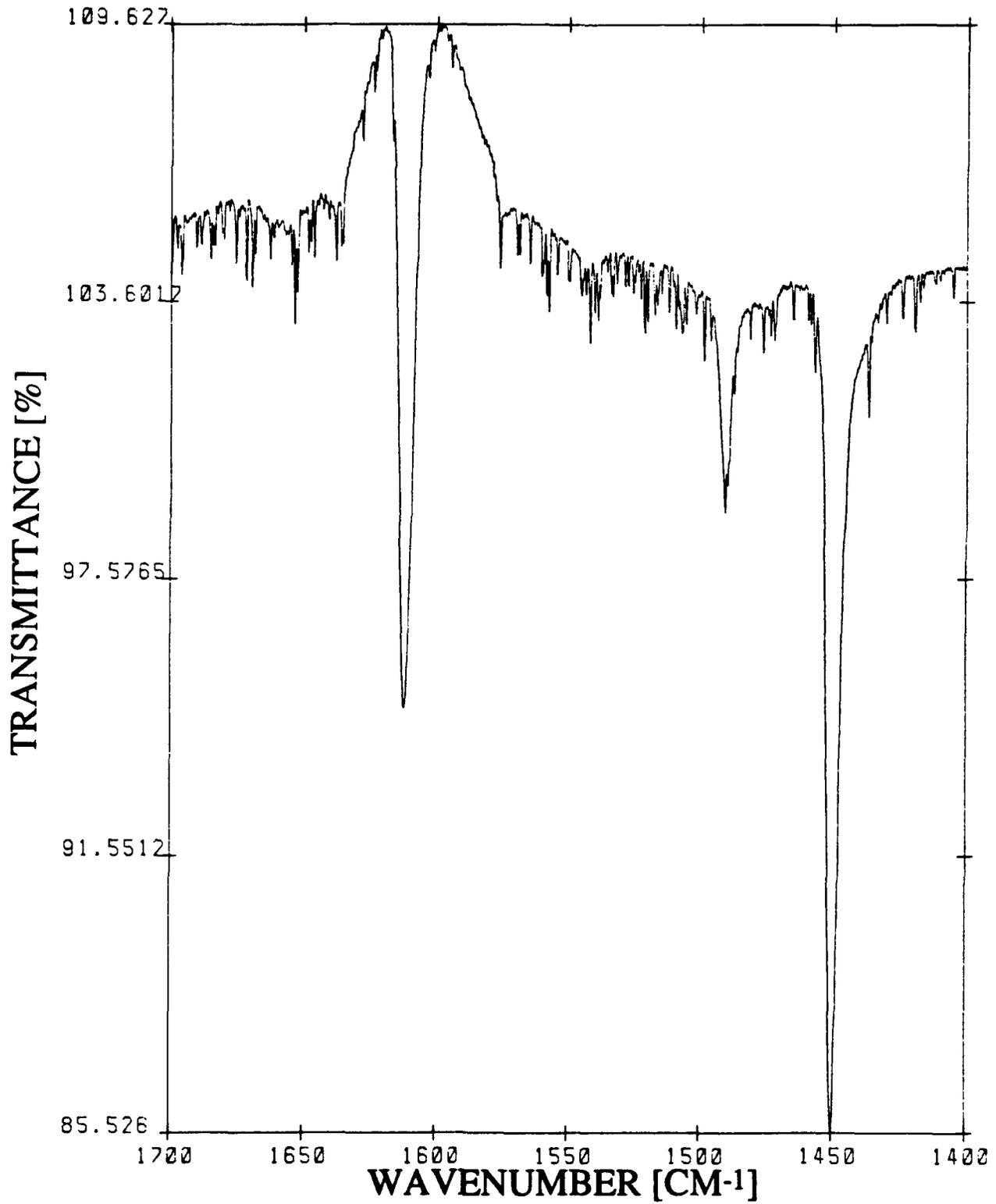
**Figure C-5:** FTIR SPECTRUM OF PYRIDINE ADSORBED ON A-NA25w AFTER HEAT TREATMENT AT 300 °C
