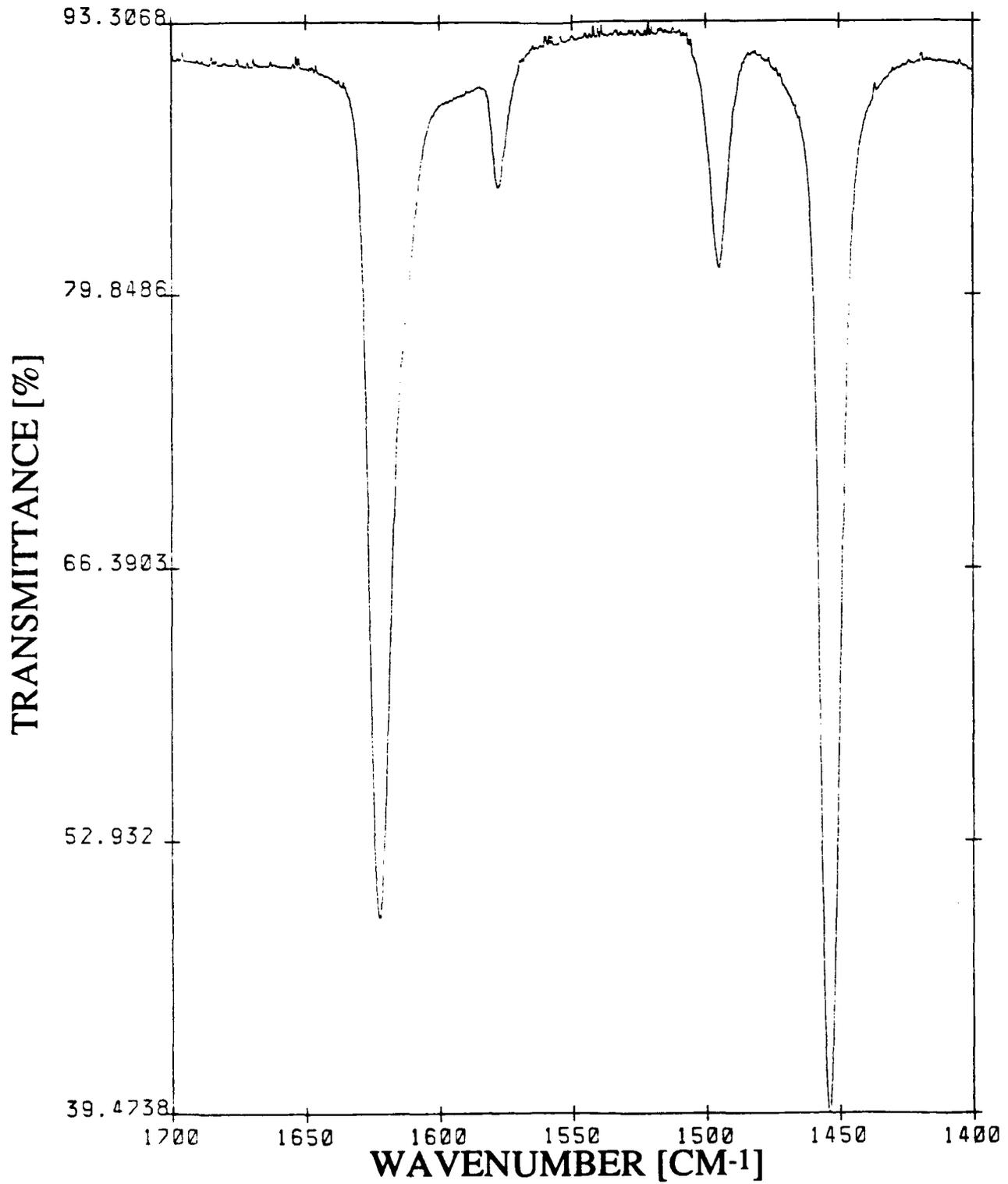
Figure C-10: FTIR SPECTRUM OF PYRIDINE ADSORBED ON A-NA(.25) AFTER HEAT TREATMENT AT 300 °C
