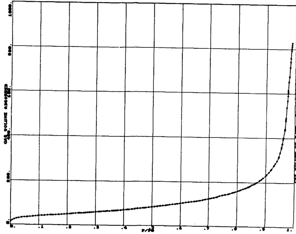
Figure B-2: PORE SIZE DISTRIBUTION FOR A-Nb<sub>2</sub>O<sub>5</sub> AS DETERMINED BY NITROGEN ADSORPTION
