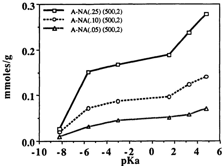
Figure 5-27: ALUMINA AEROGEL SUPPORTED NIOBIA ACIDITY (/G Nb<sub>2</sub>O<sub>5</sub>) VS. pKa
