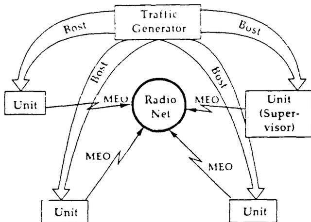
Figure 2: The relationship of the traffic generator, units, and the net resource for one net.
