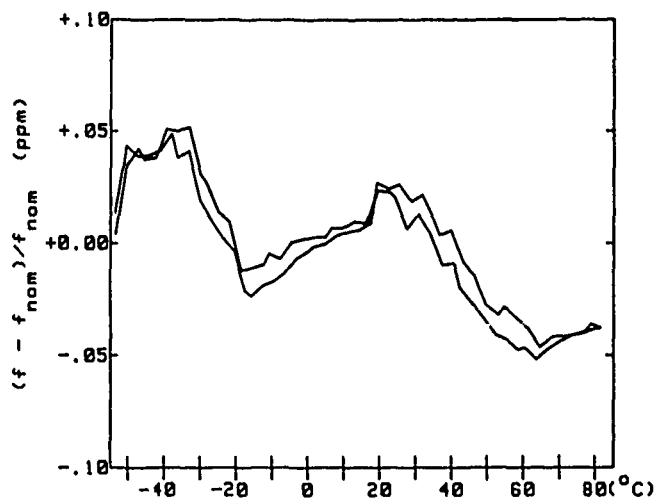
Figure 5 - f-T characteristic of MCXO 16725.
