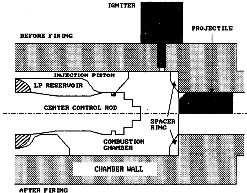
Figure 1. Concept VI Regenerative Liquid Propellant Gun.
