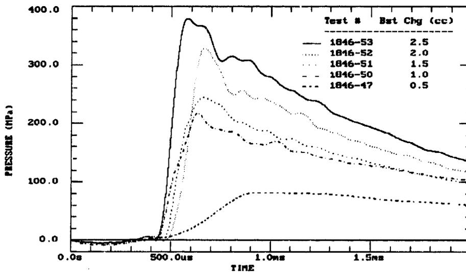
Figure 7. Filtered Antechamber Pressures.
