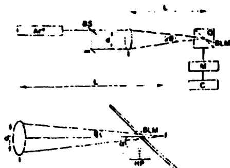
Figure 1. Schematics of the system used for observing holographic interferometry in BLMs. Ar + = argon ion laser; BS = beam splitter; m = mirror; Q = quartz cuvette; BLM = bilayer lipid membrane; M = microscope; C = camera; HP = holographic plate; f = focus; l = lens; and d = interbeam distance.
