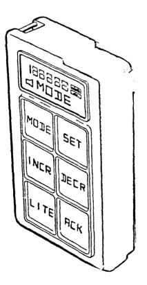
b. Pocket RADIAC Key Operations. The PR has three states of operation: "ON", "SLEEP", and "OFF".
